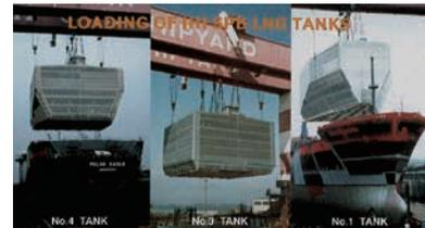
Fig. 5 IHI-SPB tanks of various shapes
