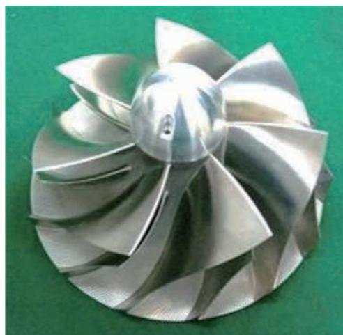
**Fig. 13** High-flow impeller used as a test piece
