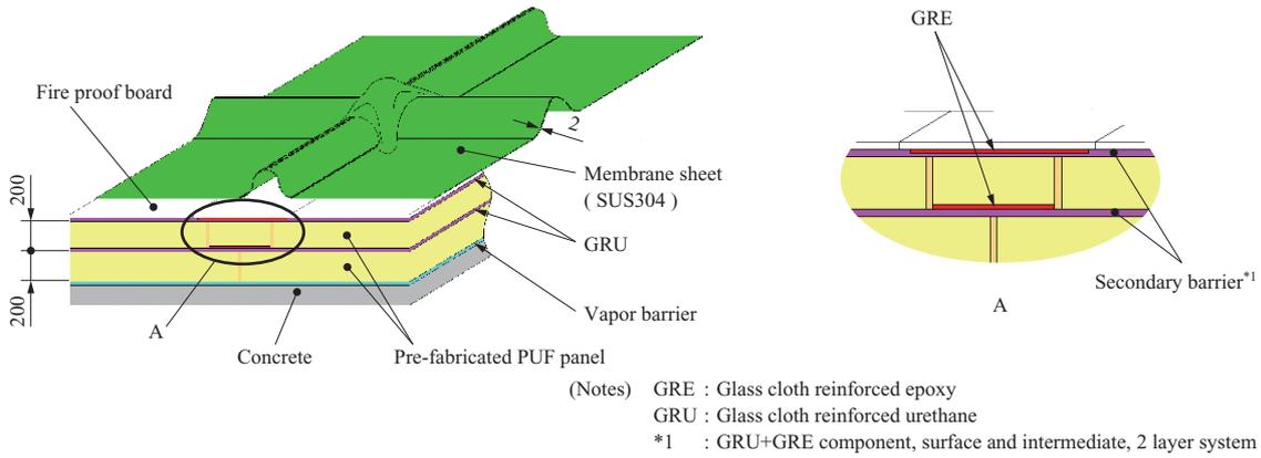
Fig. 5 Concept of secondary barrier system (unit:mm)
