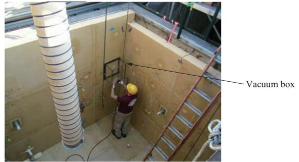
Fig. 7 Vacuum box test applied to the secondary barrier system
