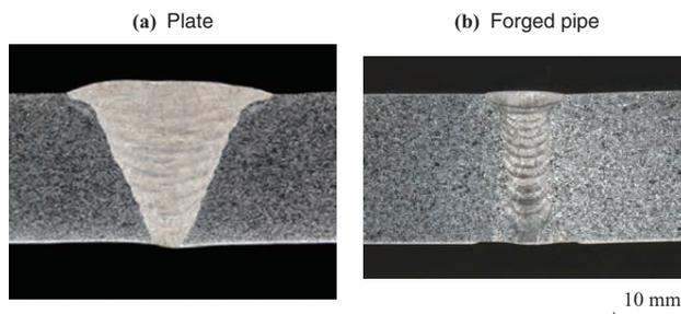
**Fig. 4** Cross-section of the macrostructure of HR6W welds
