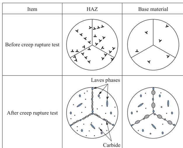
Fig. 8 Schematic illustrations showing the precipitates of HR6W welds before and after creep
