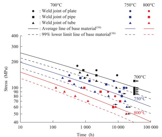
**Fig. 6** Creep rupture strength of HR6W welds at 700, 725 and 800°C at stresses from 50 to 180 MPa
