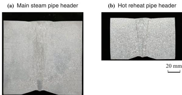
Fig. 16 Cross-section of the macrostructure of HR6W circumferential welds
