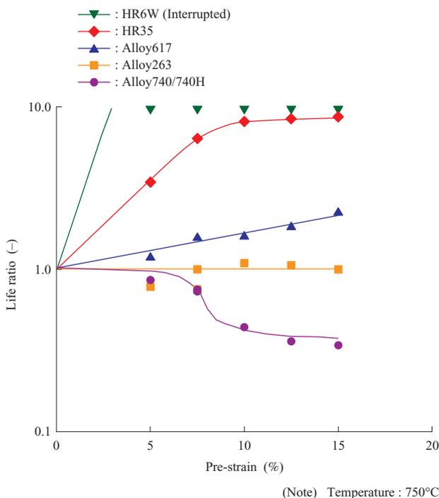
Fig. 12 The effect of cold work on the creep rupture strength of A-USC boiler tubes
