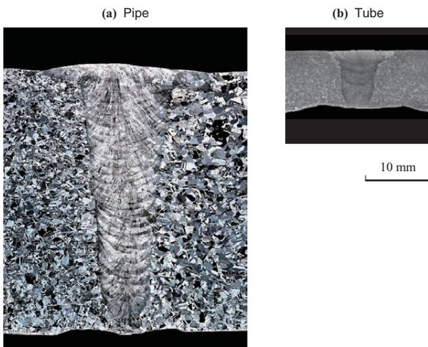
**Fig. 5** Cross-section of the macrostructure of HR6W welds
