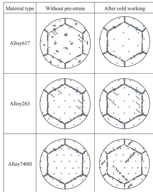
Fig. 13 Schematic illustrations showing the precipitates of cold worked Ni alloys after creep
