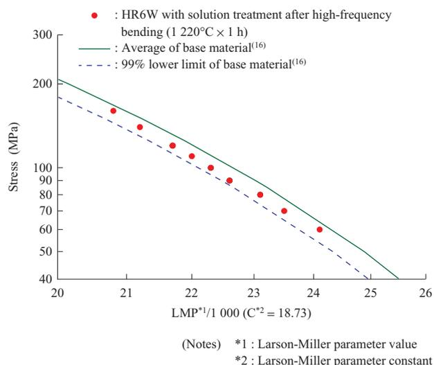
Fig. 10 Creep rupture strength of an HR6W bent pipe following the solution heat treatment
