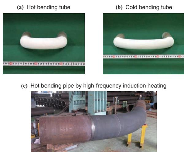
Fig. 9 Appearance of an HR6W bent pipe and tubes
