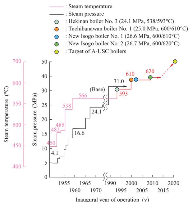
**Fig. 1** The trend in the development of steam conditions in Japan
