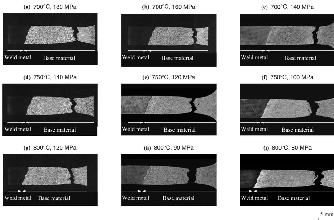
Fig. 7 Cross-sections of the macrostructure of ruptured specimens in HR6W welds
