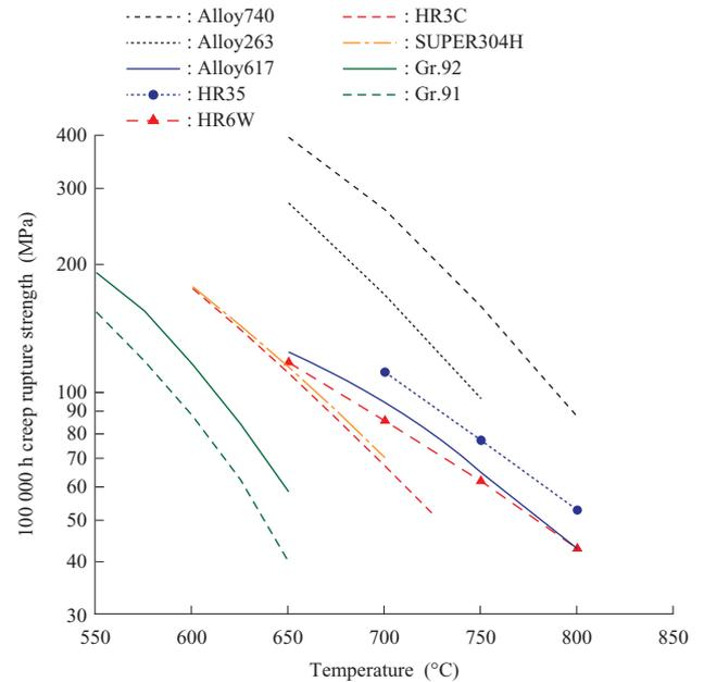
**Fig. 3** 100 000 h creep rupture strength of boiler materials
