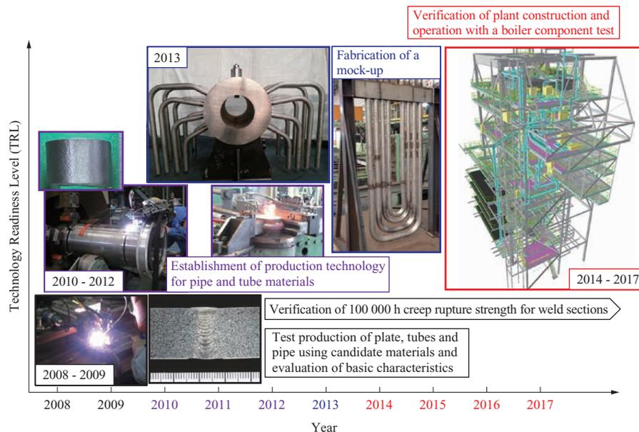
**Fig. 2** The development plan of A-USC technology
