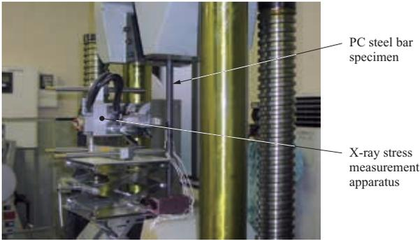
Fig. 5 Status of PC steel bar testing on a tensile machine and stress measurement by the X3000
