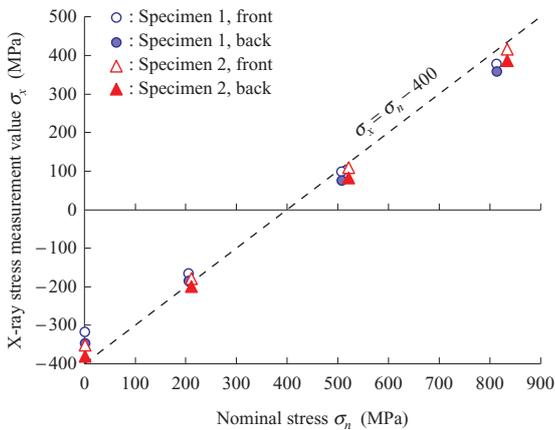
Fig. 6 Relation between nominal stress and stress measured by the X3000 in the tensile test of a PC steel bar
