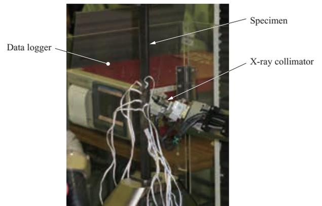
**Fig. 11** Status of the uniaxial tensile test
