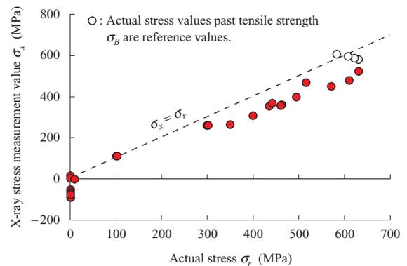
Fig. 8 Relation between actual stress ( $\sigma_r$ ) and stress measured by the X3000 ( $\sigma_x$ )
