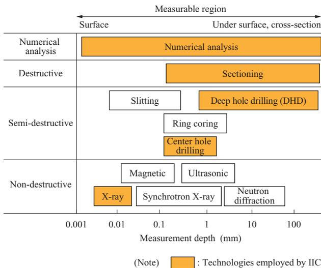
Fig. 2 Various residual stress measurement methods
