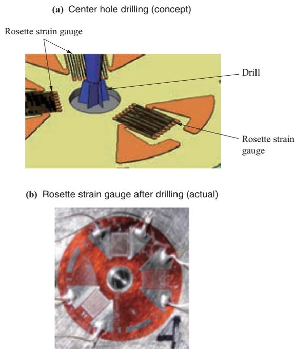
**Fig. 9** Rosette strain gauge
