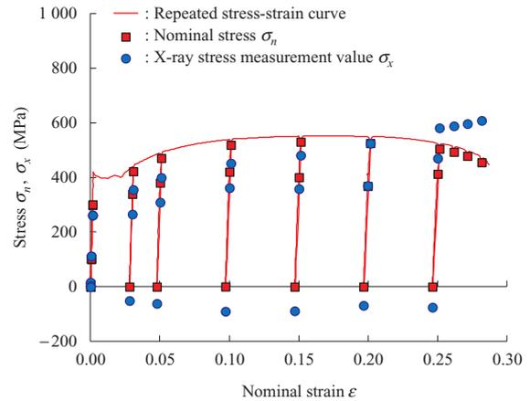
Fig. 7 Relation between strain ( $\epsilon$ ), nominal stress ( $\sigma_n$ ) and stress measured by the X3000 ( $\sigma_x$ )
