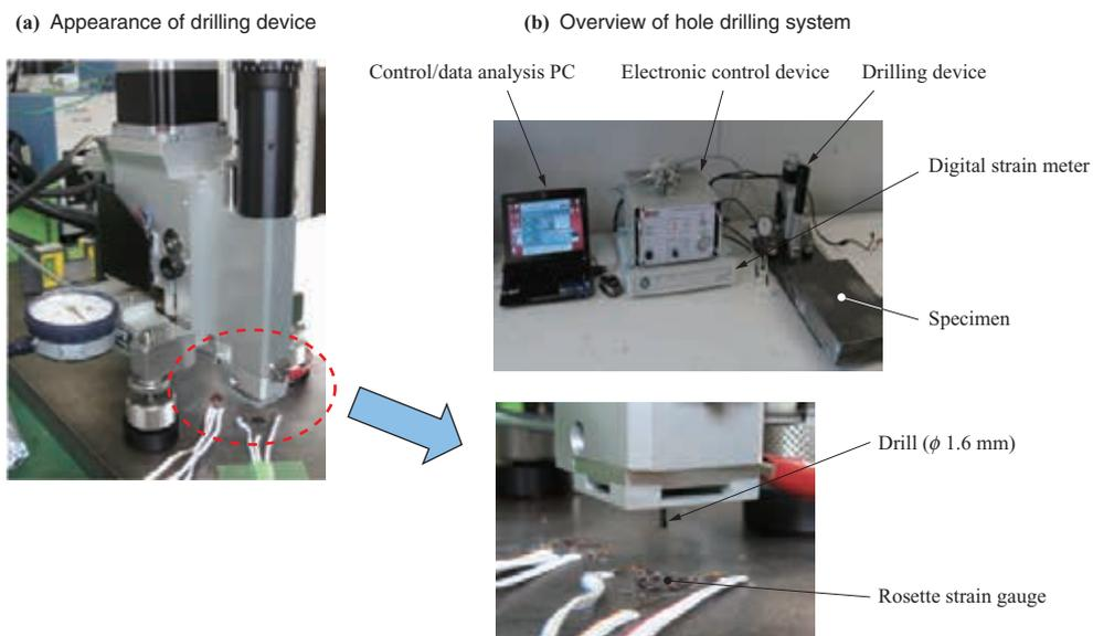
**Fig. 10** Appearance of the hole drilling system
