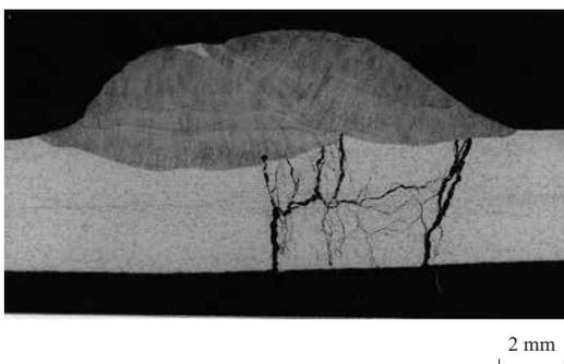
**Fig. 1** Stress corrosion crack (SCC) caused by residual stresses during the welding process
