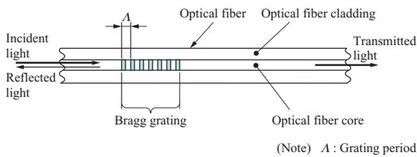
Fig. 2 Schematic of FBG principle
