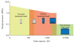
Scope of application of above-ground LNG storage tanks
