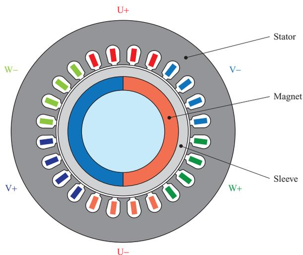
**Fig. 1** Schematic cross sectional view of the high speed motor
