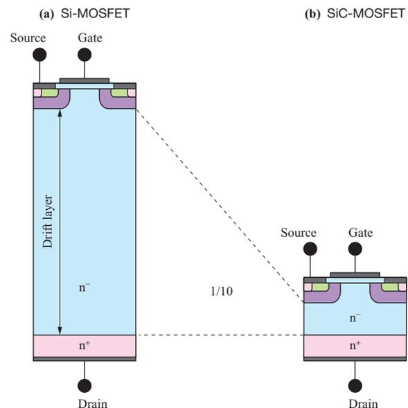
Fig. 8 Schematic cross sectional view of MOSFETs
