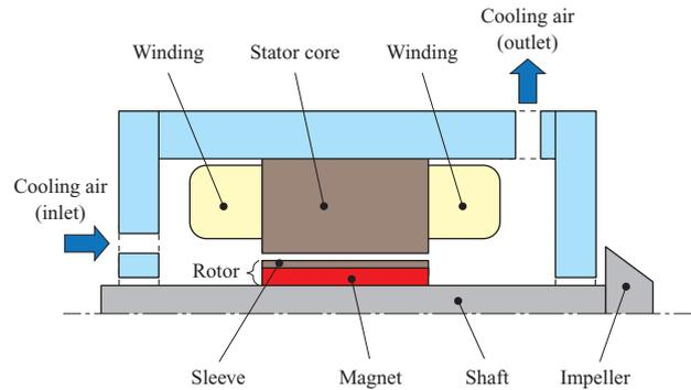
**Fig. 2** Schematic cross sectional view of high speed rotating machinery
