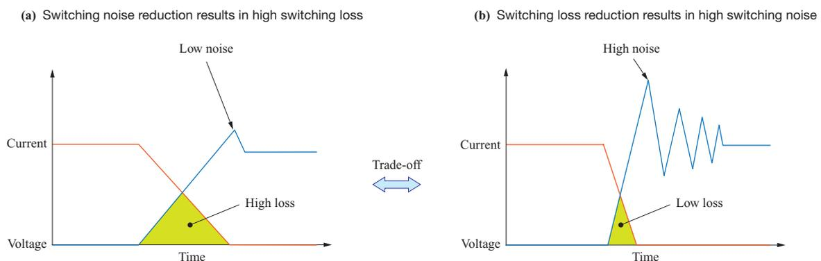
Fig. 9 Trade-off of switching characteristics
