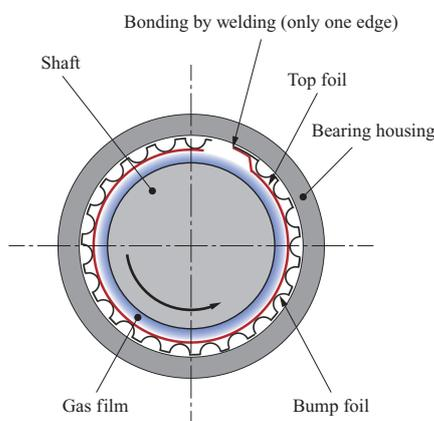
**Fig. 4** Schematic cross sectional view of foil-type dynamic radial gas bearing
