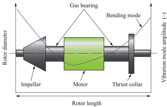
Fig. 6 Illustration of critical speed analysis
