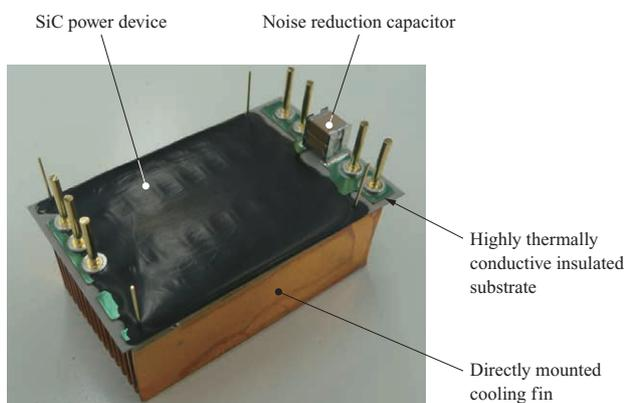
Fig. 10 Prototype of SiC power module
