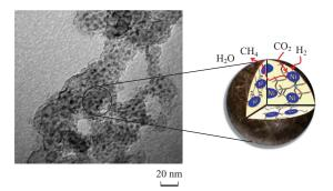
Photo and schematic of catalyst developed by IHI-ICES (reference: https://doi.org/10.1016/j.cattod.2017.03.003)
