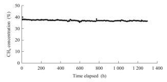
Fig. 6 Long term stability test of IHI's methanation catalyst
