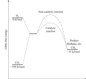
Fig. 2 Energy diagram of CO<sub>2</sub> conversion
