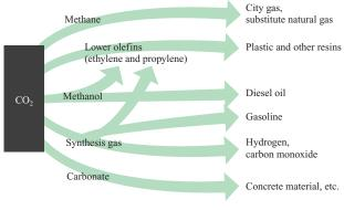
Fig. 1 Potential routes of CO<sub>2</sub> utilization
