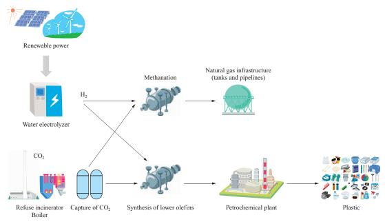
Fig. 3 Schematic process of CO<sub>2</sub> conversion to valuable products
