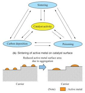
Fig. 4 Sintering of active metals on catalyst surface
