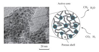
Fig. 5 TEM and schematic images of IHI Methanation catalyst
