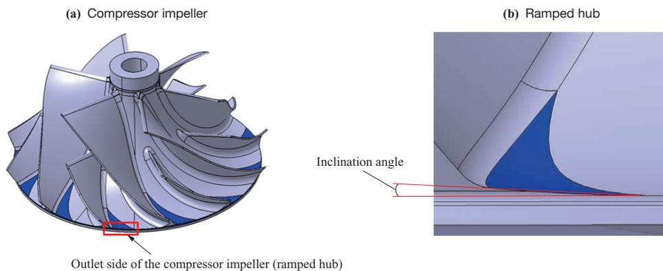
**Fig. 5** Ramped hub
