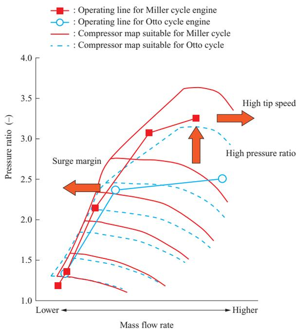
Fig. 1 Engine operating line and compressor map
