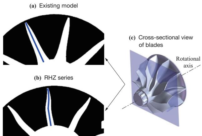
**Fig. 7** Turbine wheel cross section
