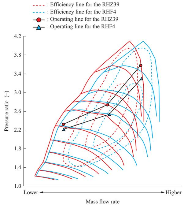
**Fig. 6** Compressor map of existing model (RHF4) and RHZ series
