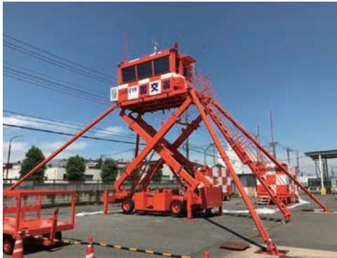
Emergency air traffic control tower system deployed for operation
