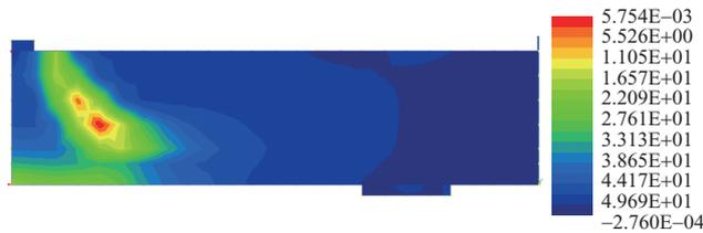
**Fig. 16** First principal strain contour at maximum load (punching shear test)
