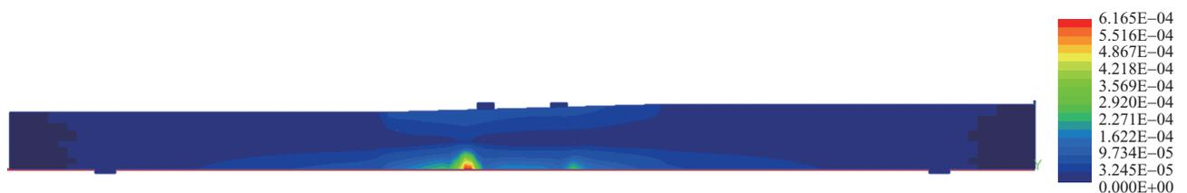
**Fig. 22** First principal strain contour (Case 1-P5, deflection : 3.0 mm)
