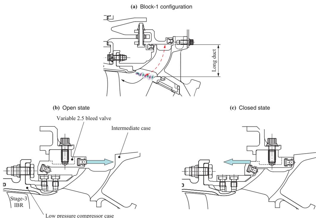
**Fig. 10** Variable 2.5 bleed valve cross-section
