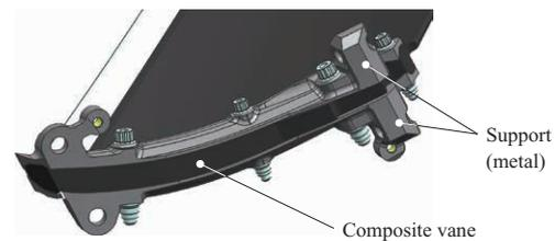
Fig. 8 Structure of composite fan exit guide vane
