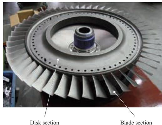
**Fig. 9** Low pressure compressor stage-2 IBR
