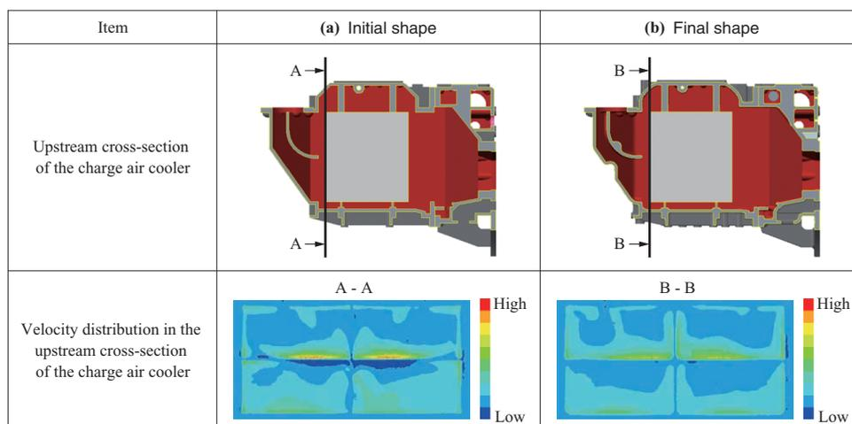
**Fig. 7** Velocity distribution in the upstream cross-section of the V28AHX charge air cooler core
