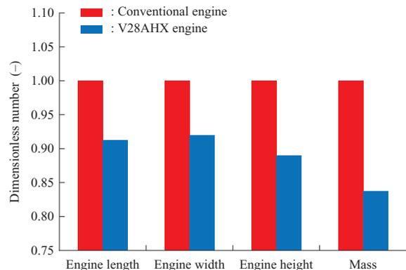
Fig. 6 Comparison of weight and dimensions between the V28AHX and NIIGATA's conventional engines
