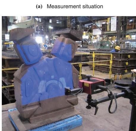
Fig. 5 3D measurement situation and measurement results of a wooden casting mold for the V28AHX engine
