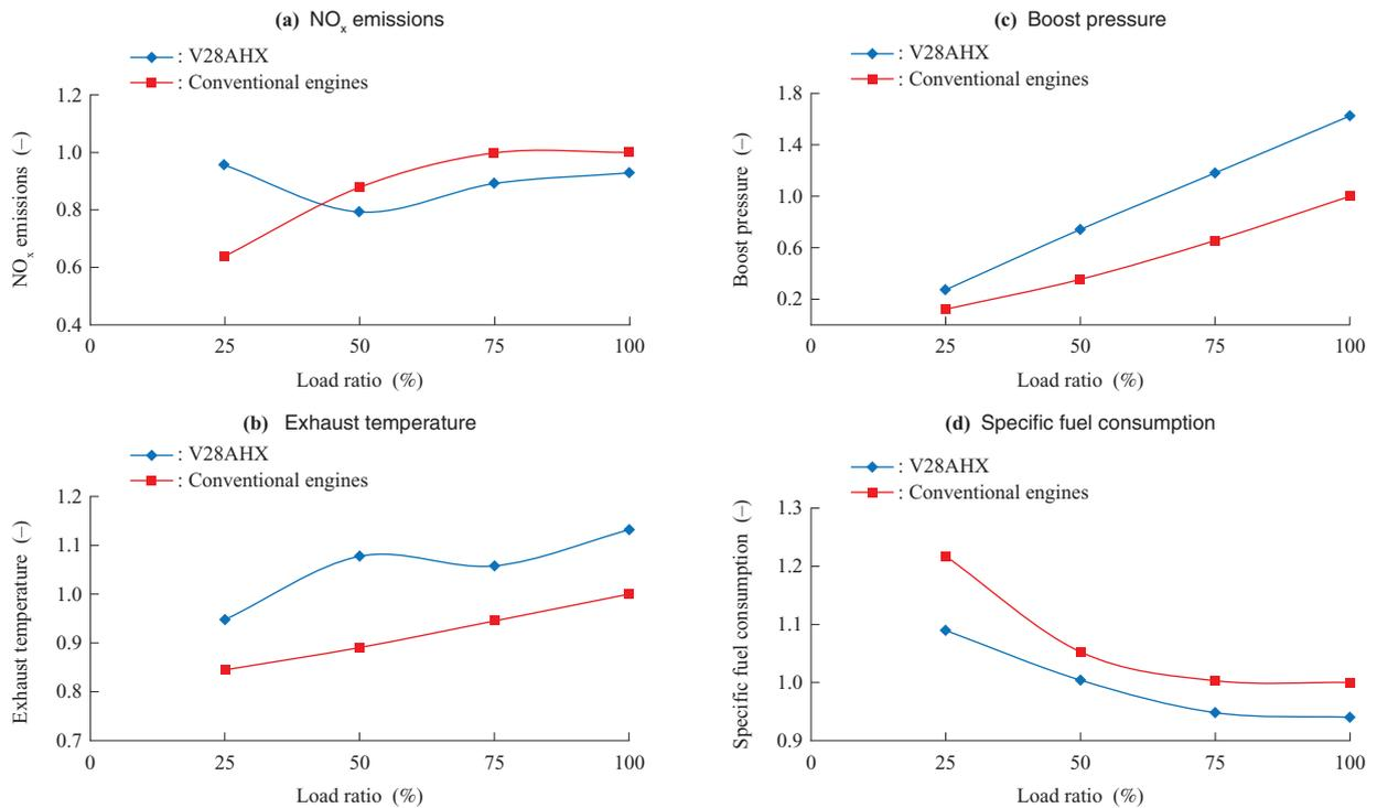
Fig. 12 Comparison of engine performance between the V28AHX engine and NIIGATA's conventional engines
