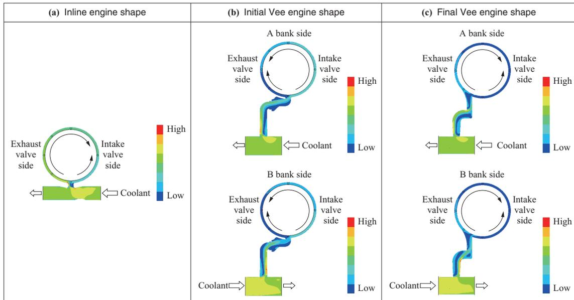
Fig. 11 Velocity distribution of coolant flow from the main coolant pipe toward the liner ring
