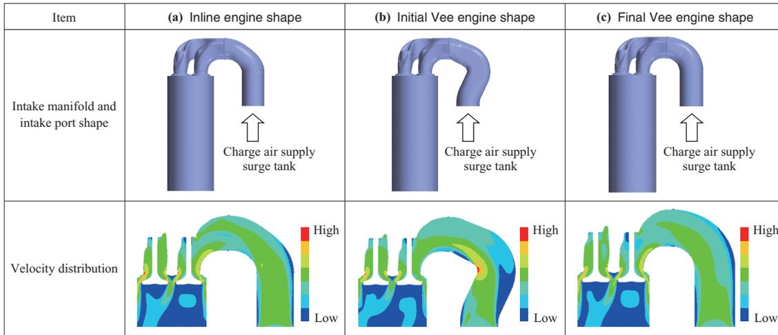
Fig. 8 Velocity distribution of the intake manifold and intake port
