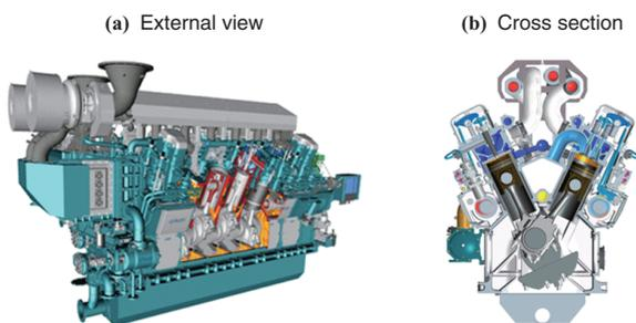
Fig. 4 External and sectional views of the V28AHX engine
