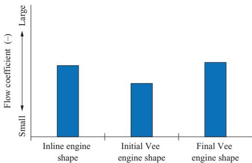
Fig. 9 Comparison of the flow coefficient of the intake manifold + intake port
