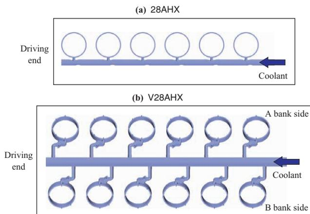
Fig. 10 Coolant circuit layout (Top view)
