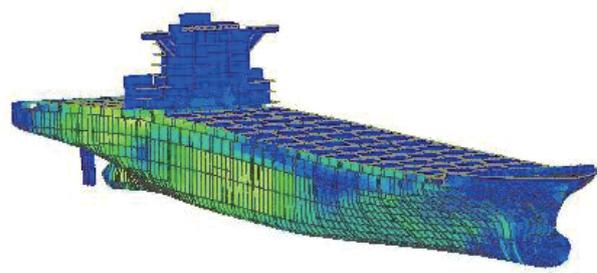
Fig. 13 Extensive structural analysis by SPB-HULL
