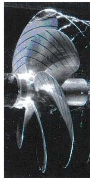
Fig. 7 Observation of propeller cavitation in cavitation tunnel
