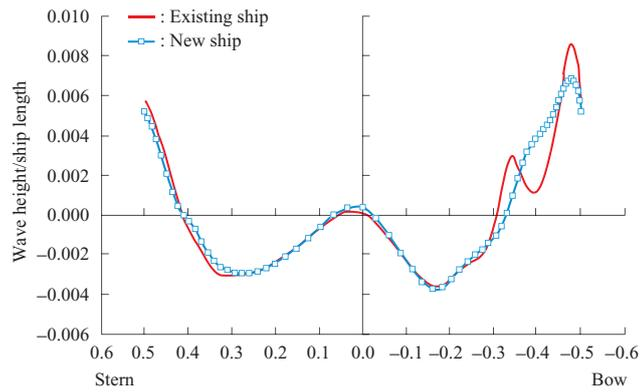
Fig. 4 Wave patterns calculated by CFD
