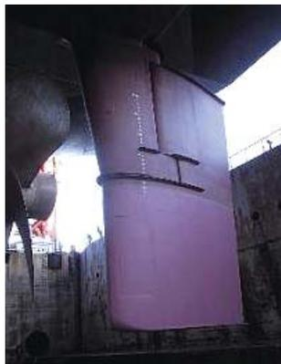
Fig. 9 Improved rudder against erosion
