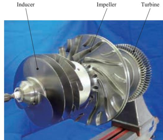
**Fig. 4** LE-9 engine fuel turbopump rotor assembly
