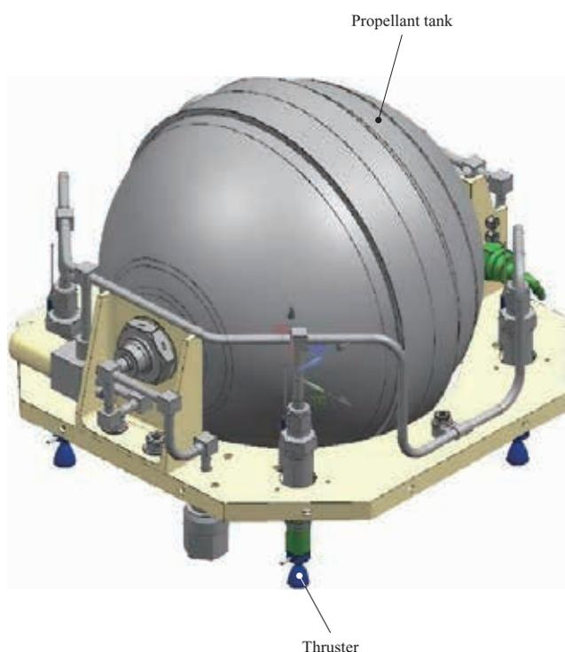
Schematic diagram of propulsion unit
