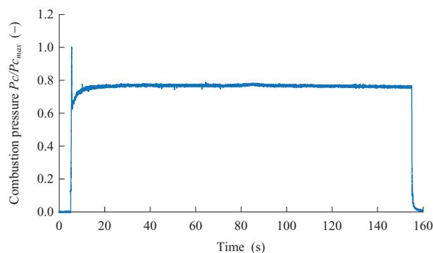
Continuous jet mode test (Combustion pressure waveform)
