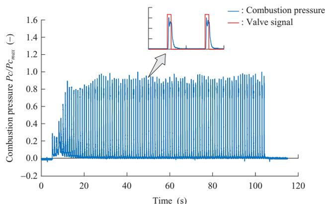
Pulse jet mode test (Combustion pressure waveform)
