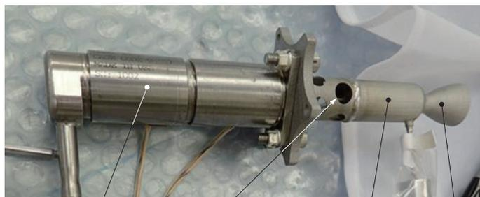
Valve      Supply piping part      Combustion chamber      Nozzle
