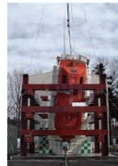
**Fig. 8** Photograph before and after the drop test (2nd test)
