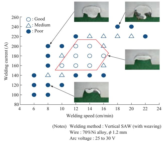
**Fig. 4** Appropriate welding condition range of vertical SAW (Flux No. 3)
