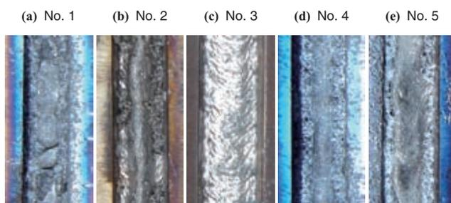
**Fig. 3** Examples of bead appearances by vertical SAW using commercial fluxes
