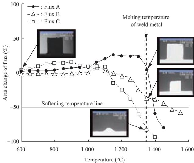
Fig. 5 Results of flux softening temperature evaluation test<sup>(4)</sup>
