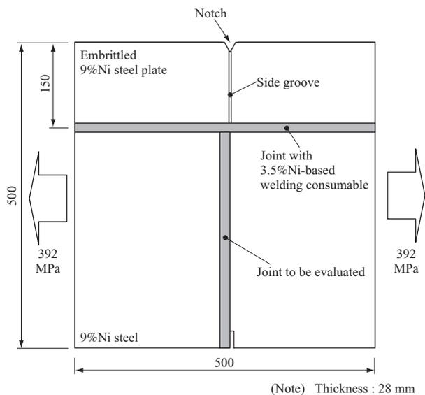
Fig. 12 Duplex ESSO test specimen (unit : mm)
