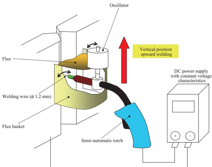
Fig. 2 Schematic illustration of vertical SAW
