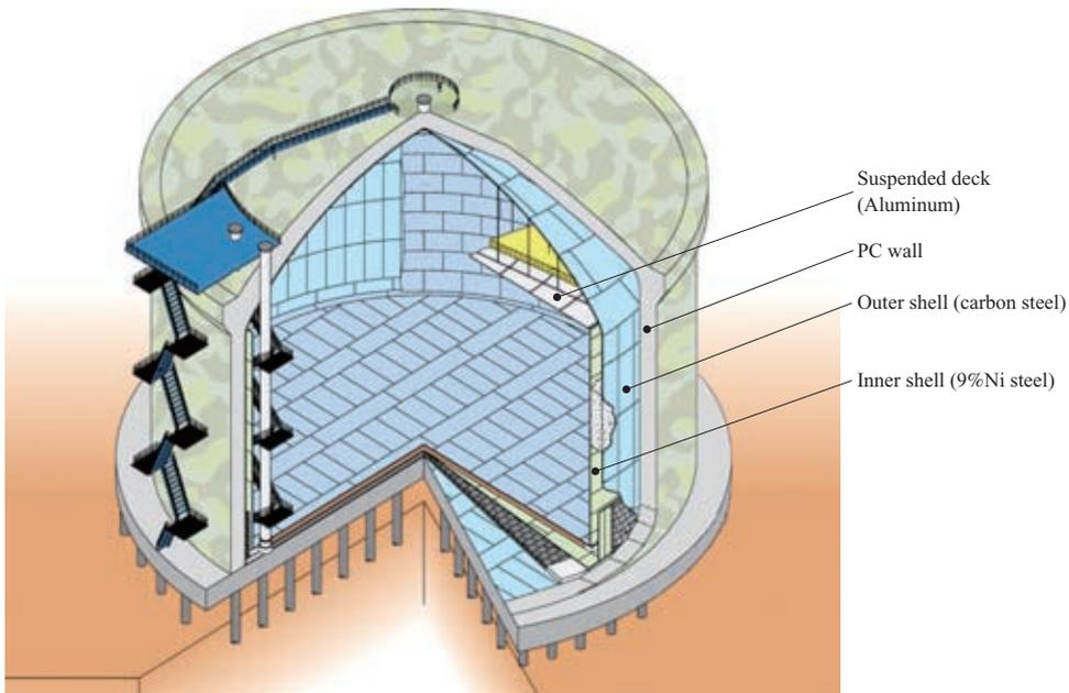
Fig. 1 Structures of PCLNG storage tank (overseas specification)
