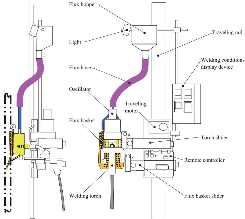
Fig. 7 Equipment for vertical SAW
