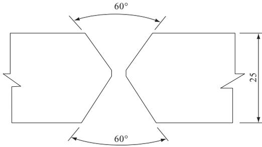
Fig. 9 Shape of X-groove (unit : mm)
