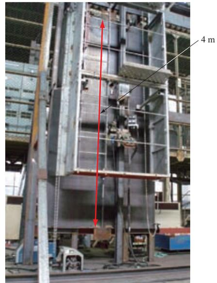
Fig. 13 Appearance of welding mock up tests with using large-size test plate (Plate thickness : 28 mm)
