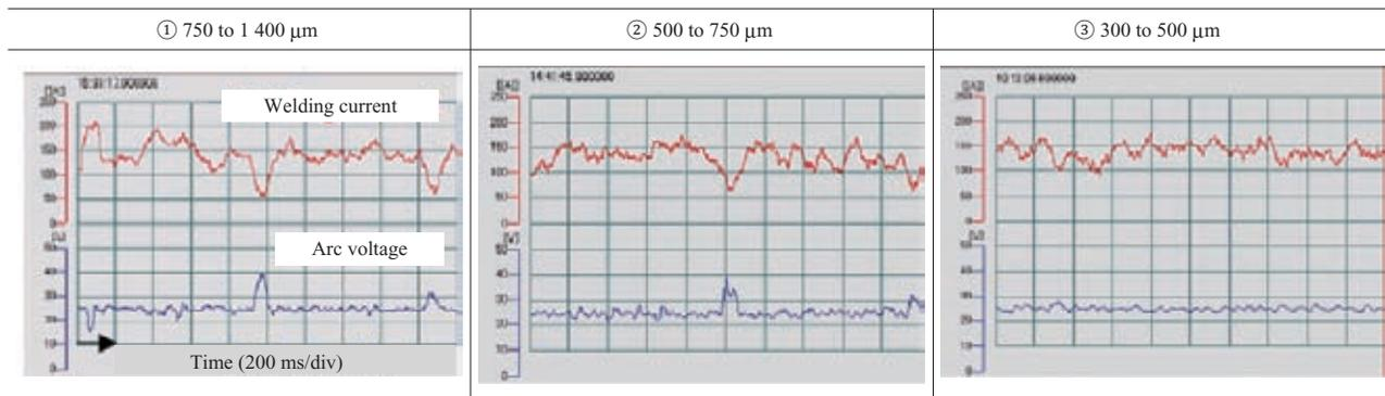
Fig. 6 Influence of particle size distribution on welding current and arc voltage<sup>(5)</sup>
