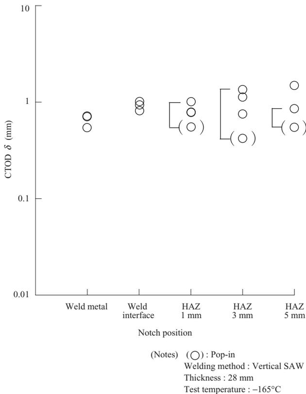
Fig. 11 CTOD values of welding joint by vertical SAW
