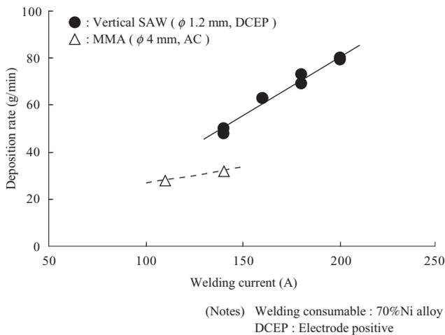
Fig. 8 Comparison of deposition rate between vertical SAW and MMA
