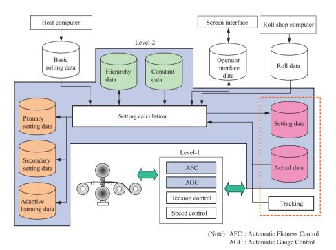
Fig. 2 Schematic chart of rolling mill setting system
