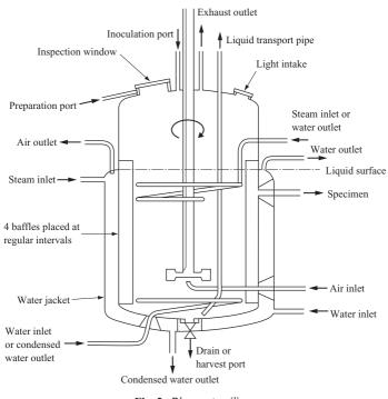
Fig. 2 Bioreactor (1)
