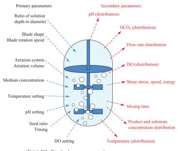
(Note) DO: Dissolved oxygen concentration DCO2 : Dissolved carbon dioxide concentration Primary parameters : Parameters that can be set by designers and operators Secondary parameters : Parameters decided by the primary parameters
