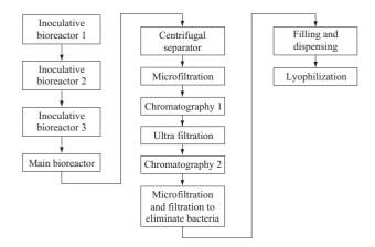
Fig. 1 Biopharmaceutical manufacturing process
