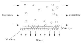
Fig. 8 Tangential flow filtration (2)
