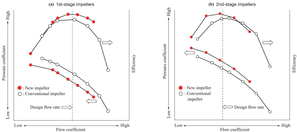
Fig. 9 Impeller performance
