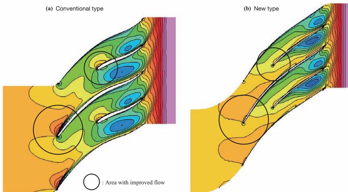
Fig. 8 2nd-stage compressor impeller relative Mach number distributions at shroud section
