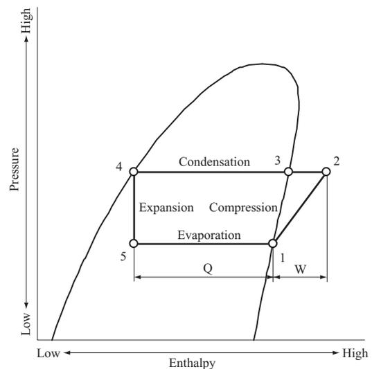
Fig. 1 Chiller heat cycle
