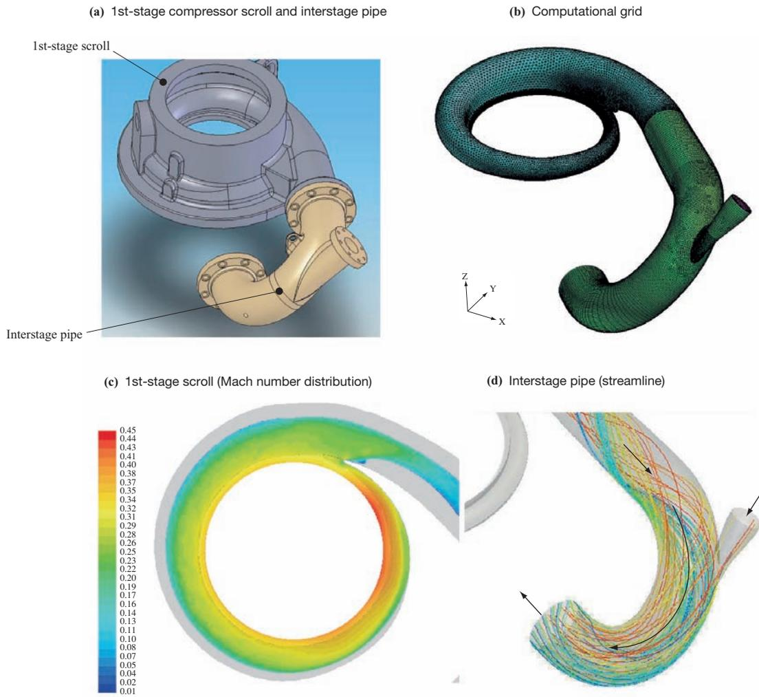
Fig. 12 CFD results of 1st-stage compressor scroll and interstage pipe
