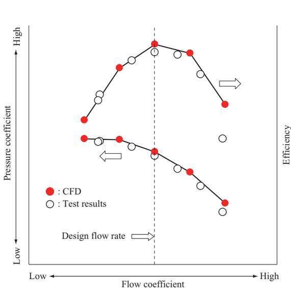
Fig. 10 1st-stage compressor performance ( comparison between CFD and test results )
