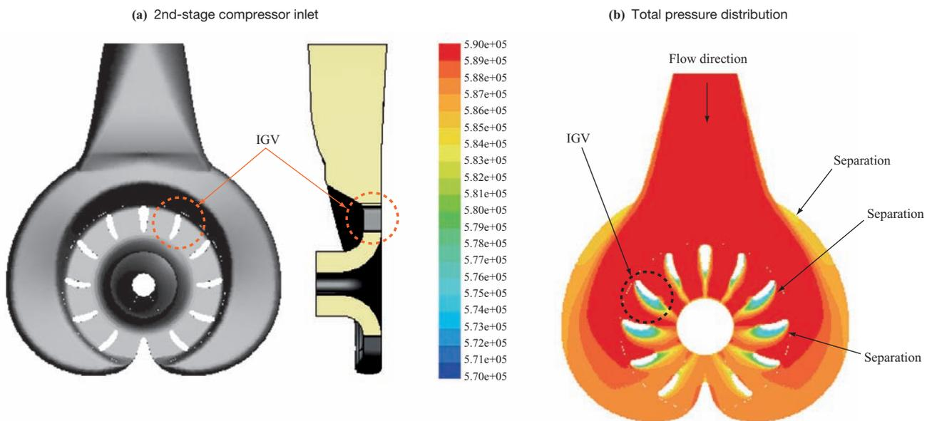
Fig. 13 CFD results of the 2nd-stage inlet
