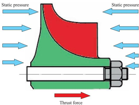
Fig. 6 Pressure force on compressor axial load
