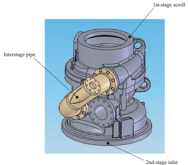
Fig. 11 Connecting conditions of the 1st- and 2nd-stage compressors
