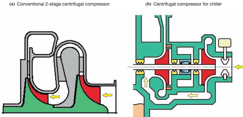
Fig. 5 Impeller arrangement of 2-stage centrifugal compressor
