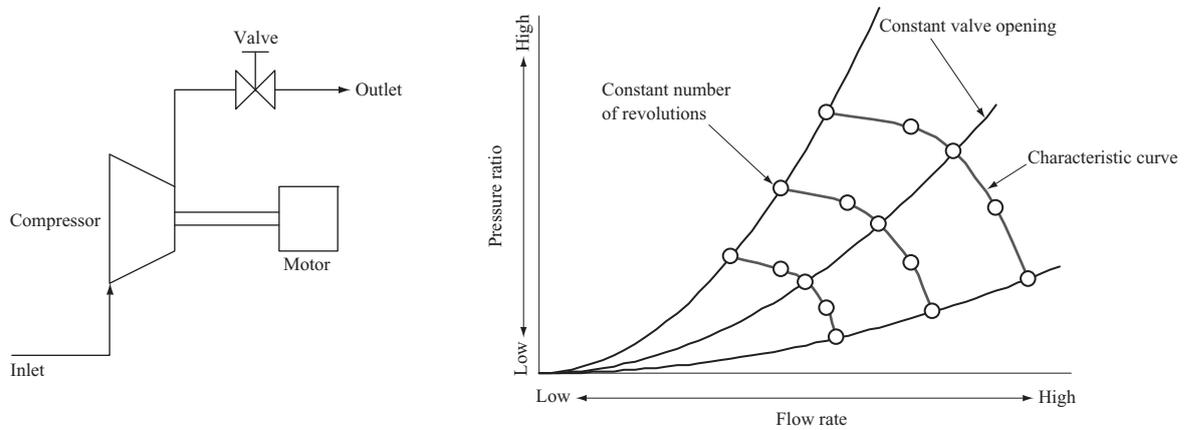
Fig. 3 Schematic of turbo-compressor test facility and compressor characteristics
