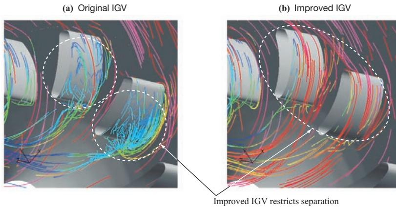
Fig. 14 Streamline around IGV in the 2nd-stage inlet
