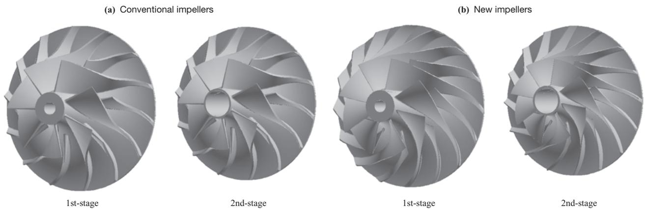
Fig. 7 Conventional and latest impeller shapes
