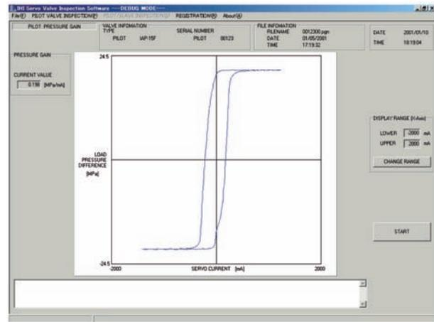
**Fig. 10** Characteristics of pressure gain of pilot valve
