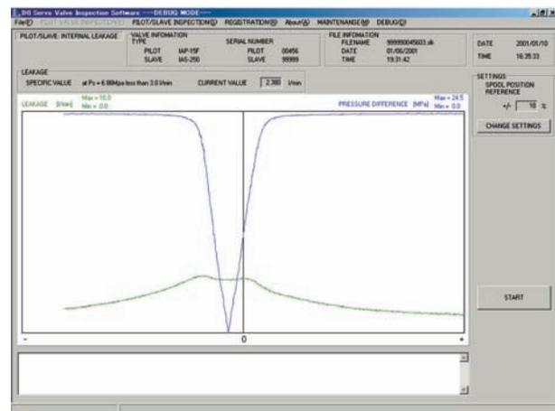
**Fig. 11** Characteristics of internal leakage of combined valve
