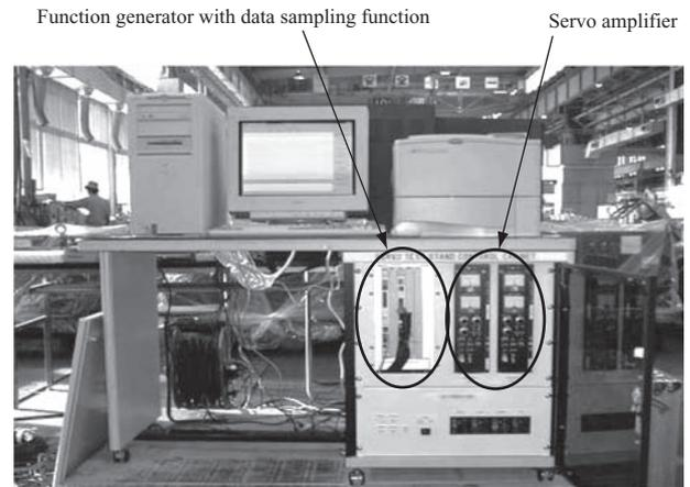
Fig. 8 Control system equipment
