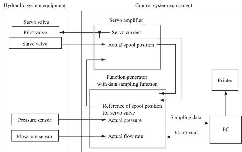
Fig. 6 Configuration of servo valve diagnosis system
