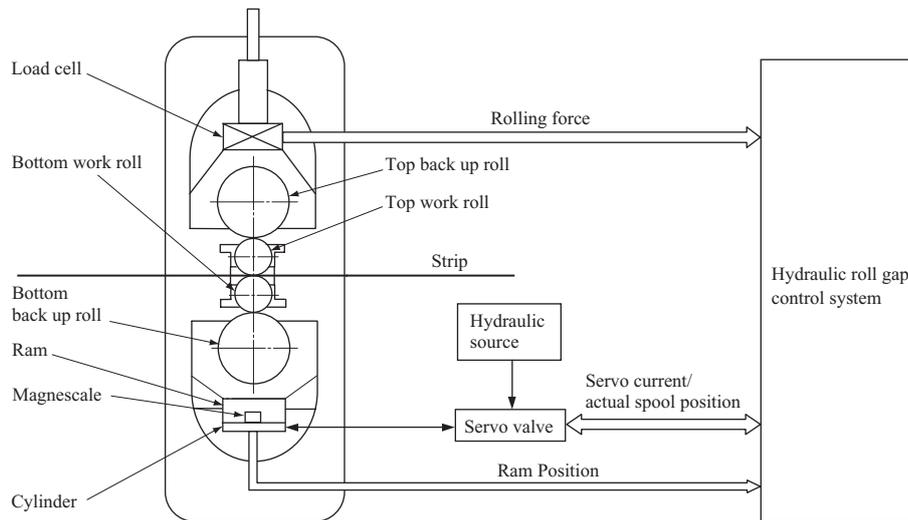
Fig. 1 Configuration of hydraulic roll gap control system
