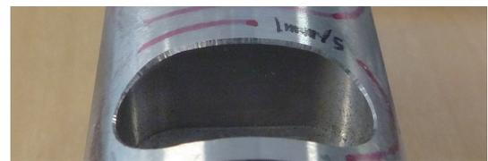
**Fig. 12** Overview of chamfered edge : Slot on a cylinder
