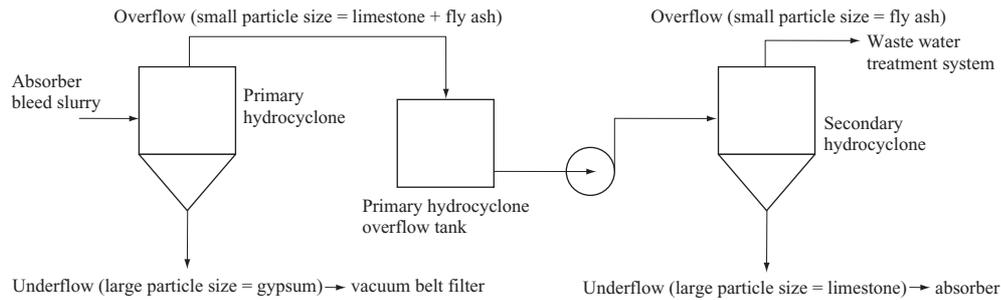
Fig. 6 Principle of two-stage hydrocyclone classifier
