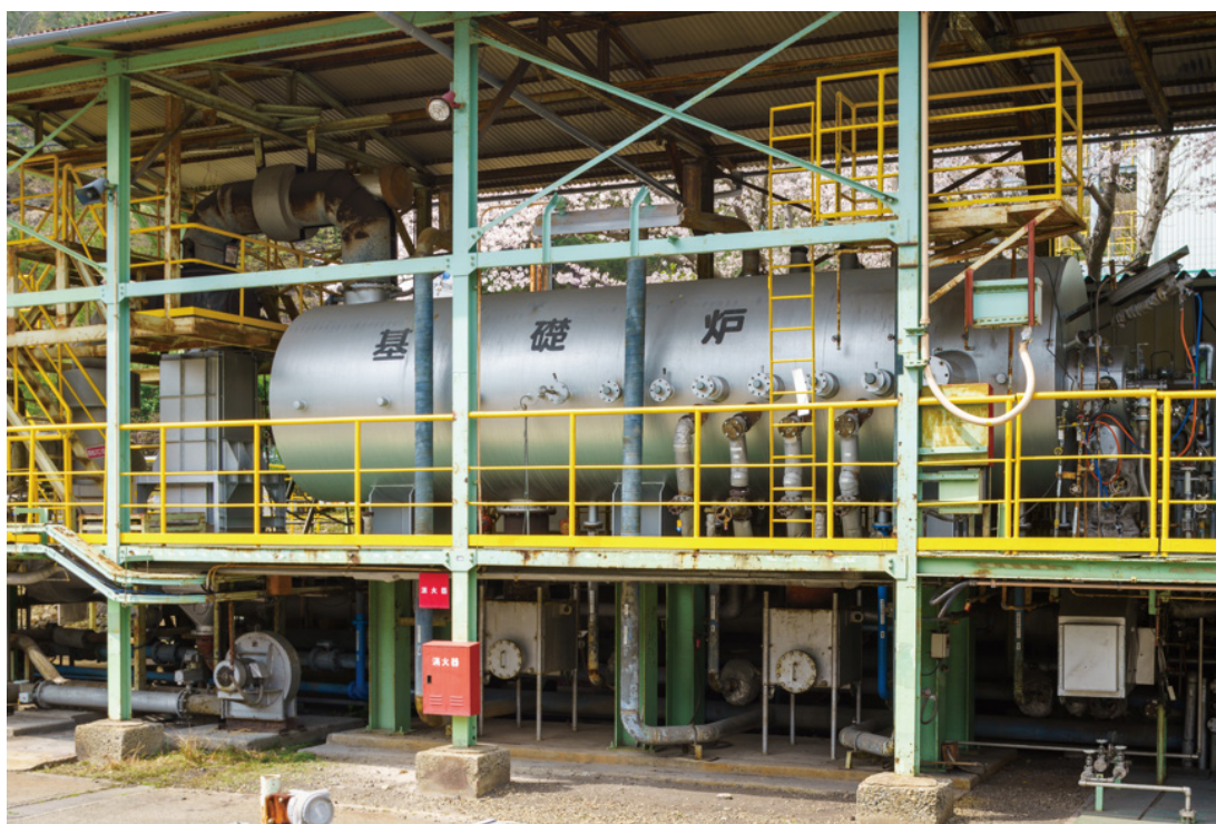
Basic combustion test furnace at the D&D Park in the IHI Aioi Works
