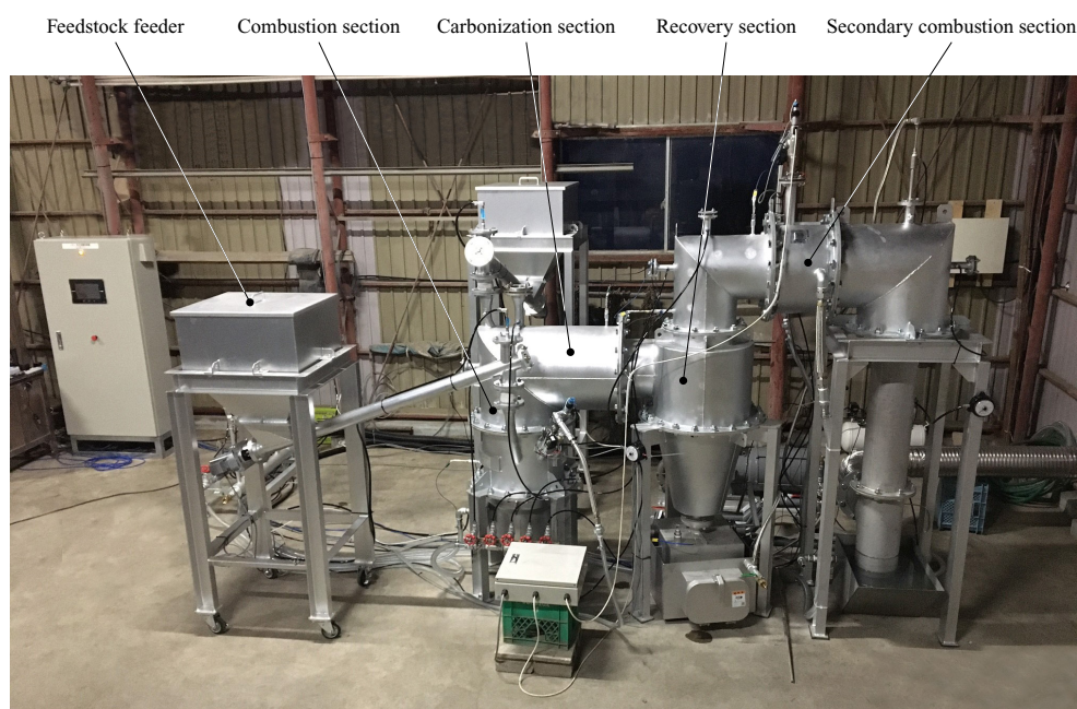
High-speed carbonization method with partial combustion (2 t/d prototype machine)
