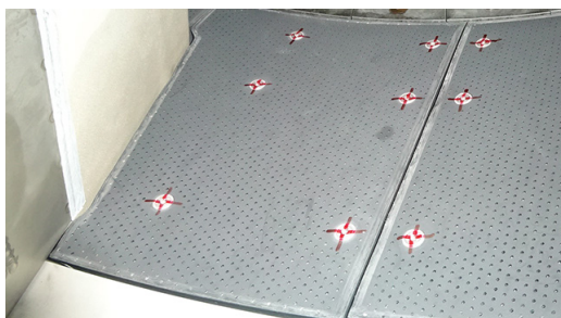
Fig. 8 Resin-based acoustic liner mounted on the JAXA F7 engine
