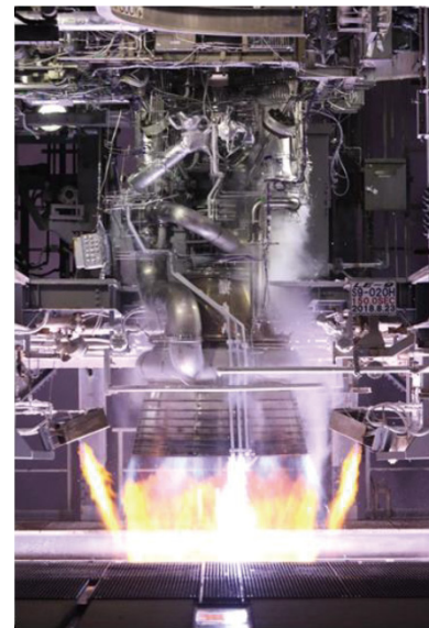
Fig. 9 LE-9 engine hot firing test (4)
