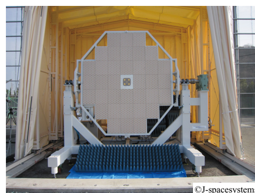
Fig. 1 Exterior view of the receiving unit for long-distance power transmission and reception demonstration test (3)
