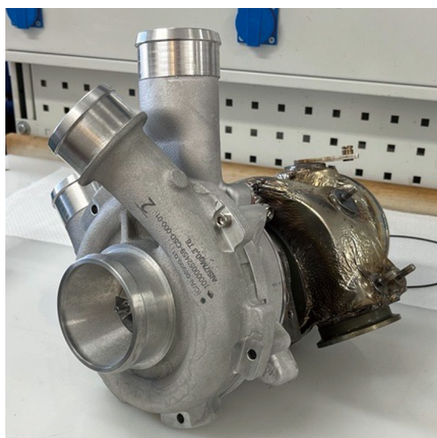
(a) Turbine driven automotive turbocharger with merged wheel setup instead of a conventional compressor stage
