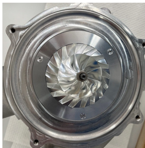
(b) View to the merged wheel compressor with the housing removed
