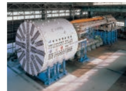
Large-diameter shield tunneling machine
