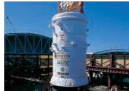
Reactor pressure vessel for BWR nuclear power plant
