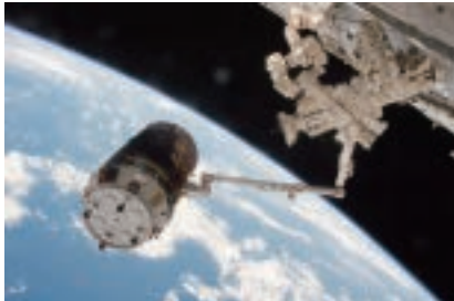
HTV propulsion system and exposed palette (HTV: H-II Transfer Vehicle) (© JAXA/NASA)
