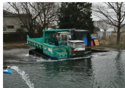
A remotely controlled heavy carrier robot at semi-underwater environment (UGV)
