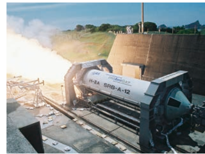
SRB-A Ground Combustion Test (© JAXA)
