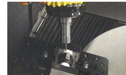
Adaptive machining from the integration of measurement and machining
