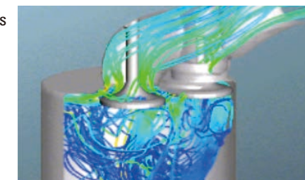
Flow analysis inside engine cylinder
