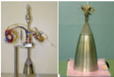
22N thruster 500N apogee engine Development of bipropellant liquid apogee engine, etc., used to obtain geostationary orbit
