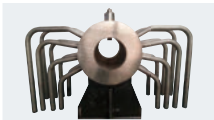
Mockup of the SH header for A-USC boiler
