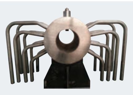
Producing mock-up for A-USC boiler application
