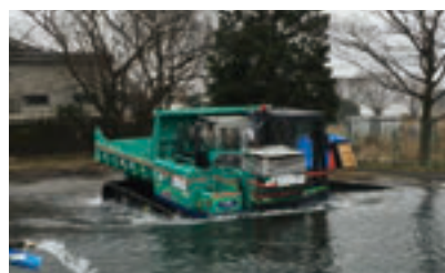
A remotely controlled heavy carrier robot at semi-underwater environment (UGV)
