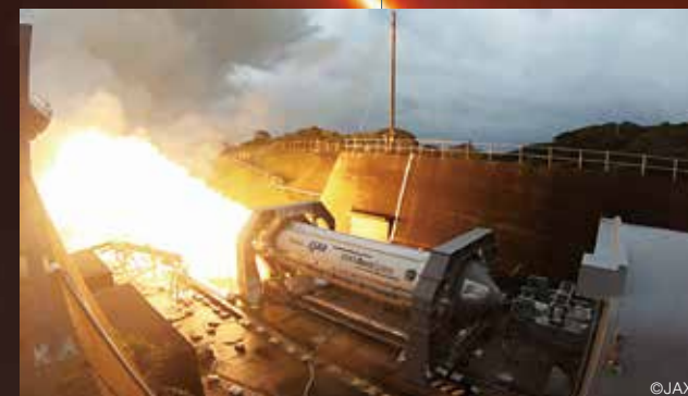
SRB-3 Ground Firing Test (QM2)
