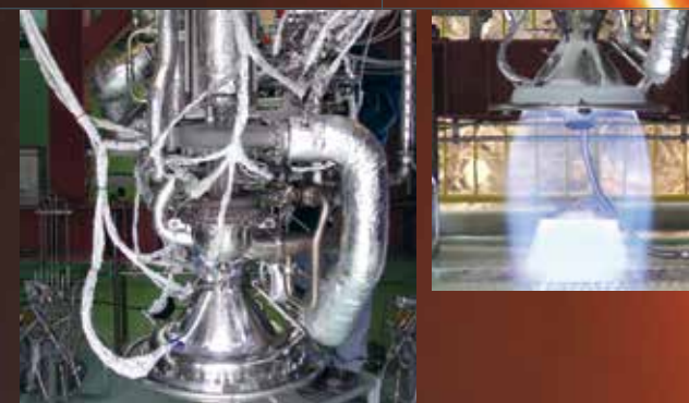
100kN Class Regenerative Cooling Meta-Engine Combustion Test
