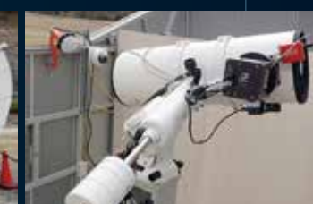
Aperture 200mm, Viewing angle 2.6 degrees, Cooling CCD camera Observation of the 120-degree longitude width of the geostationary orbit zone
