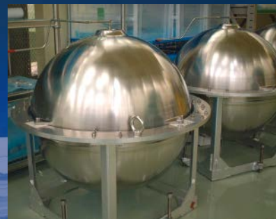
552 L tanks for HTV
