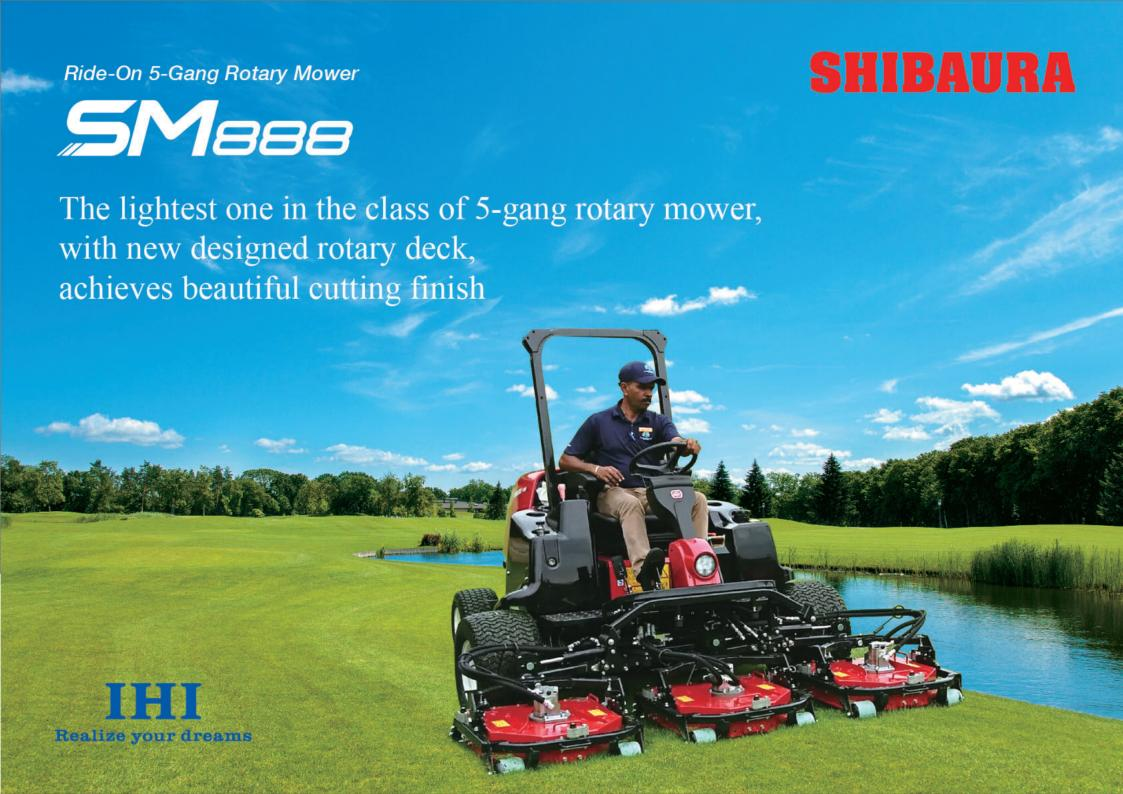
Climbing power and driving performance have been improved by the drive system "SMD" that applies Shibaura's tractor technology. "SMD" also helps save maintenance costs and reduce the risk of oil leaks.
