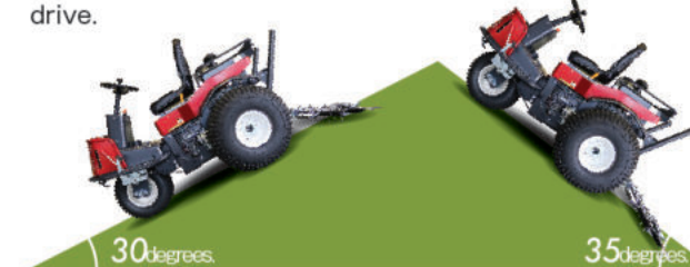
Front tipping angle: 30 degrees (tire slip)
