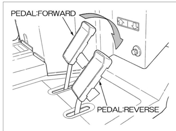
Press forward pedal down to drive the vehicle forward and the reverse pedal to reverse it. No clutch pedal is provided on this machine. Speed is increased or decreased by the amount the pedal is depressed.
