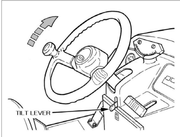
Angle of the steering wheel can be adjusted. Position of the steering wheel can be adjusted by pulling the tilt lever. After the position is determined, pull down the tilt lever forward and fix. Do not adjust these functions while the vehicle is traveling.
