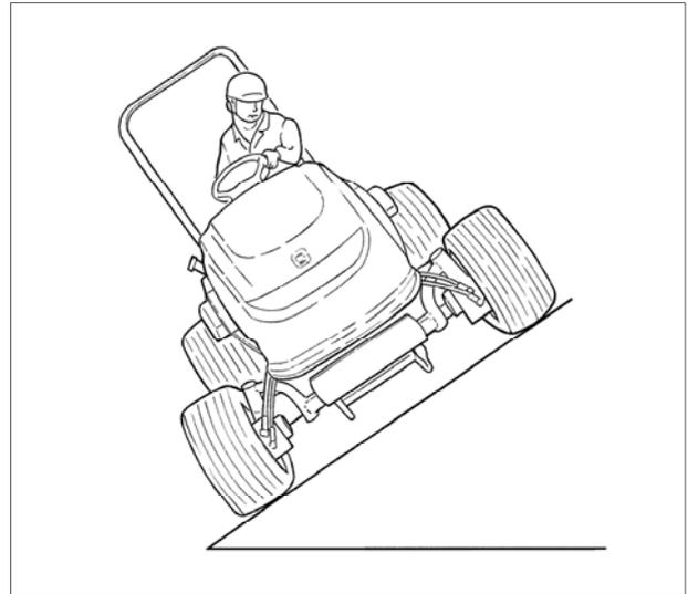
By grasping the seat swing lever above the oil tank, the seat rolls laterally in 2 steps to 12.5 and 15°. Continuous operation along the slope allows safe operation at a comfortable position.
