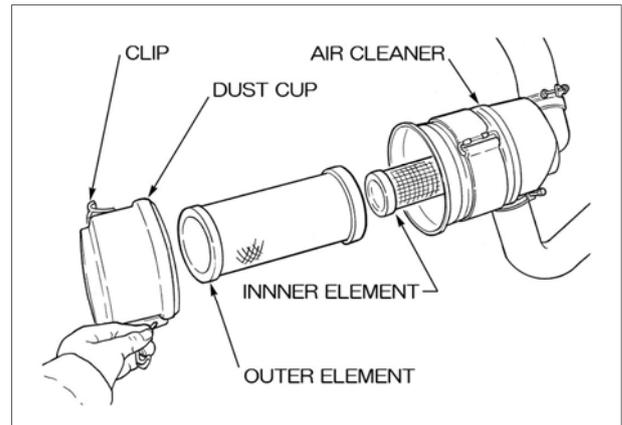
Clean the outer element every 100 hours and replace it after cleaning 6 times. If the operation is carried out in a place subject to excessive dust, clean the air element at a shorter interval. Replace the element about once a year even though the specified interval has not been expired.
