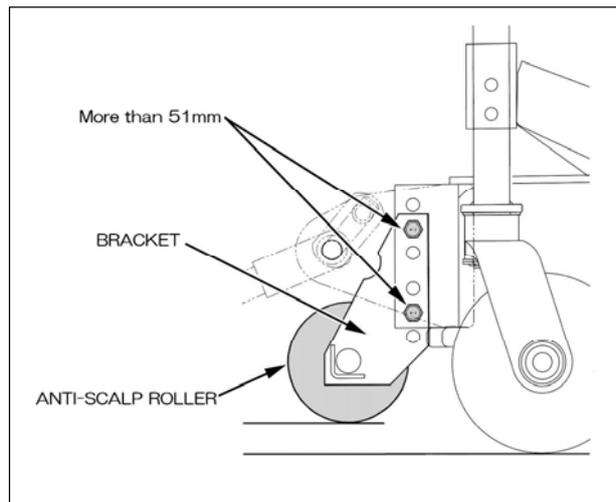
When you set cutting height as 51 mm or more, please fix with an attached bolt nut in the hole above a bracket, and the hole below a mower.
