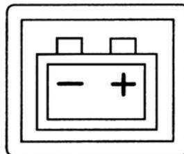
When the main switch is turned to the “ON” position, the lamp lights up. After the engine starts, number of engine revolutions increases. When charging is started, the lamp goes out.
