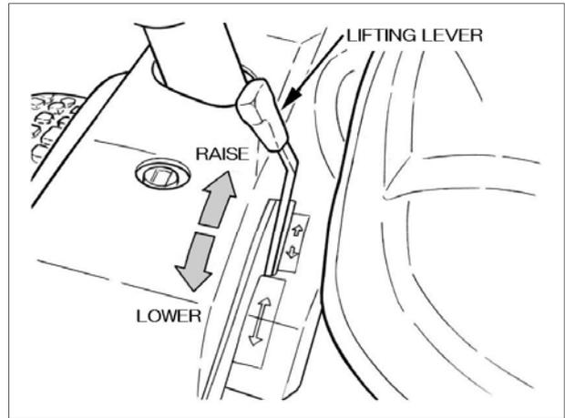
By pushing down the lever rearward, the mower rises. When you release your hand from the lever, it automatically returns to the neutral position. By setting the lever to the lowering position, the lever is held at the lowered position and the mower becomes free to float over undulating ground.
