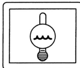
Even though the main switch is turned to the “ON” position, the lamp does not light up. The lamp lights up if the engine is overheated during operation. In such a case, stop the operation and check the cause.
