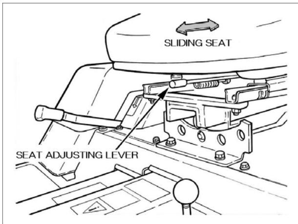
The seat slides forward and backward. Release the seat by movement of the lever. Adjust the seat properly to your operating position.
