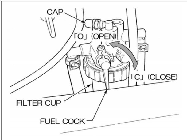
The fuel feed pump of this machine is driven from the cam shaft. After it is operated for cleaning or replacement, remove the cap and discharge the air in the filter cup.
