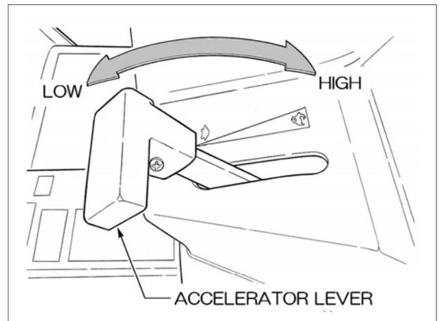
The accelerator lever is used to increase or decrease the engine revolutions. By pulling the lever toward the operator, the engine revolutions decrease and by pushing it forward, the engine revolutions increase.
