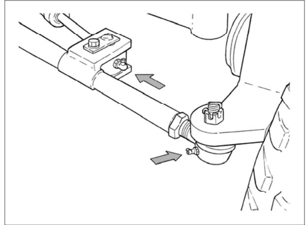
Power steering cylinder (at 2 points), tie rod end (2 points)
