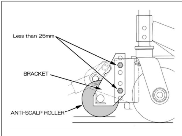
When you set cutting height as 25 mm or less, please fix with an attached bolt nut in the hole of the bracket bottom, and the hole above a mower.
