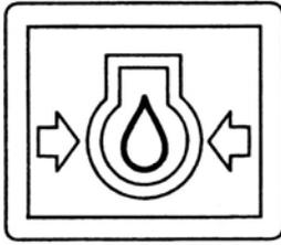
When the main switch is turned to the "ON" position, the lamp lights up. When the engine starts operation, the lamp goes out. If the lamp lights up while the engine is rotating, there is a fault in the lubrication pressure circuit. Stop the engine immediately and check for the trouble.
