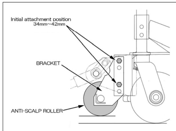
When cutting height sets to 34 mm - 42 mm, please fix with an attached bolt and nut in the hole above a bracket, and the hole above a mower. (Initial attachment position)
