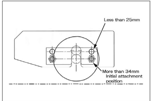
When cutting height is 34 mm or more, please fix a bracket in a lower position. (Initial attachment position)
