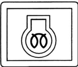
By setting the main switch to the "Glow" position, the lamp lights up indicating that the power is supplied to the heater. Keep the switch at the "Glow" position for about 5 seconds and then turn it to the "START" position to start the engine.
