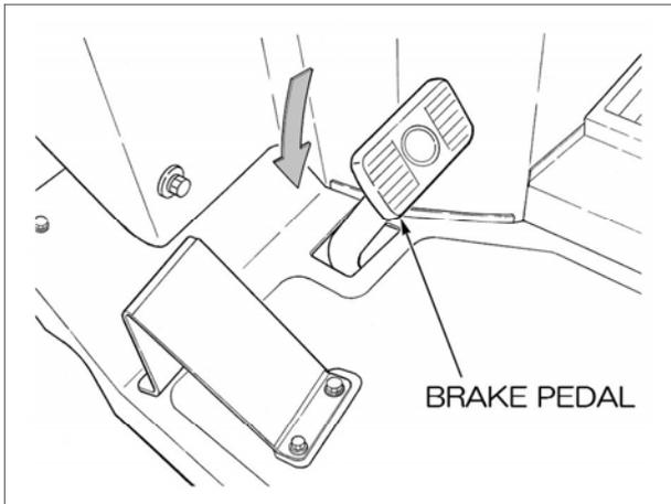
By pressing the brake pedal, brake is applied. A safe starting device is provided. Be sure to press the brake pedal when starting the engine.
