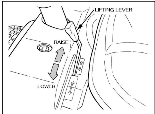
When lifting or lowering the mid mower, push the lifting lever forwards to lower the mower, and push it to the rear to lift the mower. When you leave your hand from the lever, it automatically returns to the neutral position.
