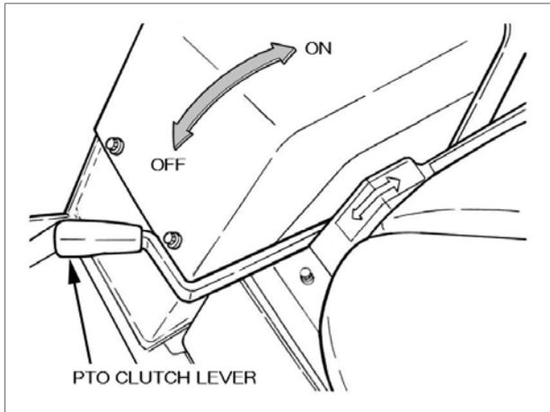
By moving the PTO clutch lever to “ON”, the blades rotate. By moving the PTO clutch lever to “OFF”, the clutch is disengaged and the blade stops rotating.
