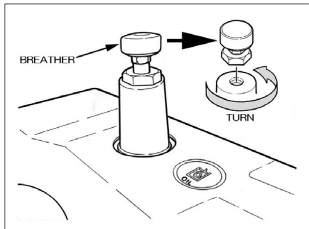
Turn the breather counterclockwise to remove it. After supplying oil, tighten the breather.
