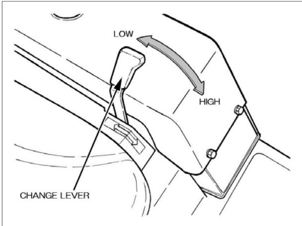
Vehicle speed can be selected from “L” (low speed) (4 WD) and “H” (high speed) (2 WD). By pushing the lever forward, the speed increases and by pushing it rearward, the speed decreases. Keep the lever on the low speed side for usual operation and use the high speed side only when traveling. When changing the speed, stop the vehicle.
