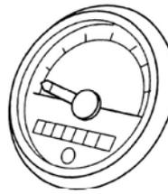
While the engine is running, its number of revolutions is indicated by the pointer. The elapsed time integrator indicates the time by a number for which the machine was operated. By multiplying the white number on the right by 6, time in the minute unit is obtained.
