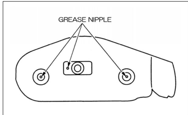
Supply grease to the idler pivot and right and left front gauge wheels every 50 hours.
