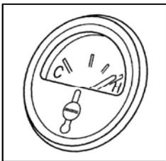
Temperature of cooling water is indicated by a pointer during operation. When the pointer points to the "H" position, engine may be overheated. Stop operation even when the engine water temperature meter lamp does not light up and check for the cause.
