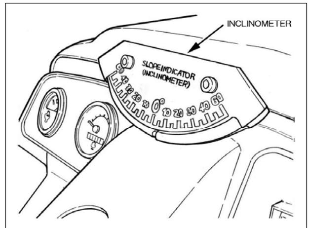
The inclination of vehicles is shown. It is not used at 25 degrees or more.
