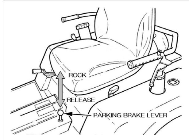
By pressing the brake pedal fully and pulling up the lever, the parking brake is applied.
