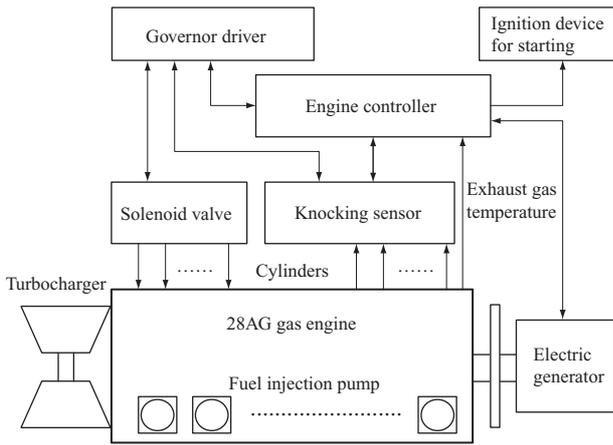
Fig. 4 Engine control block diagram
