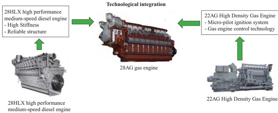
Fig. 1 Development process of 28AG engine
