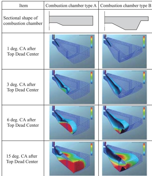
(Note) Temperature distribution : the light blue surface is isothermal surface at 1 000 K
