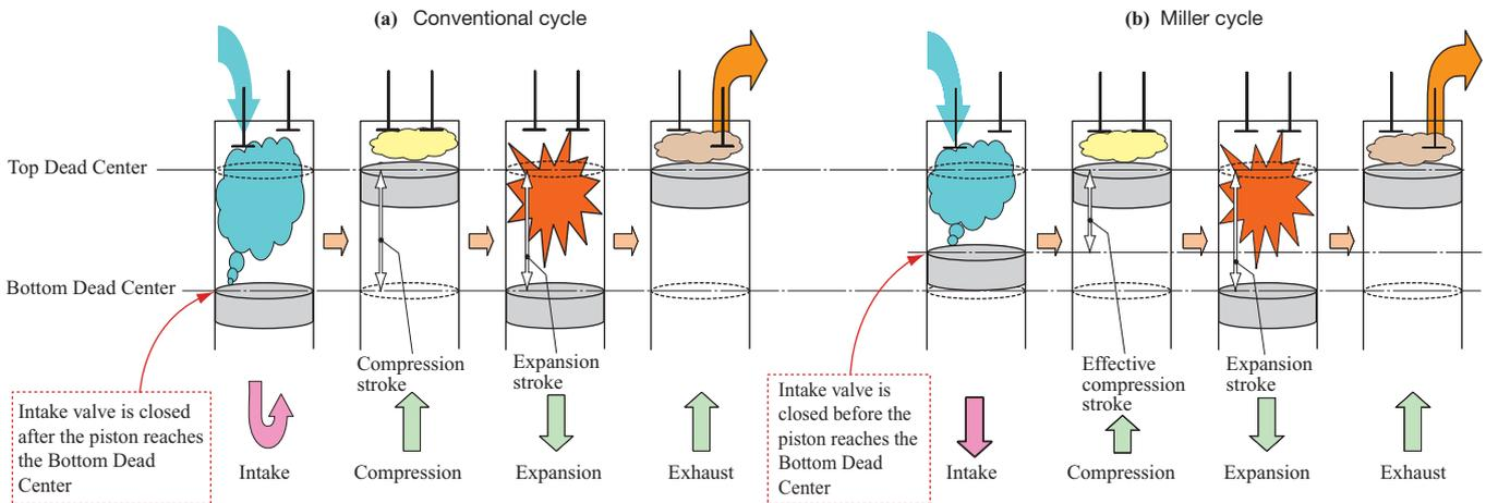
Fig. 5 Miller cycle principle
