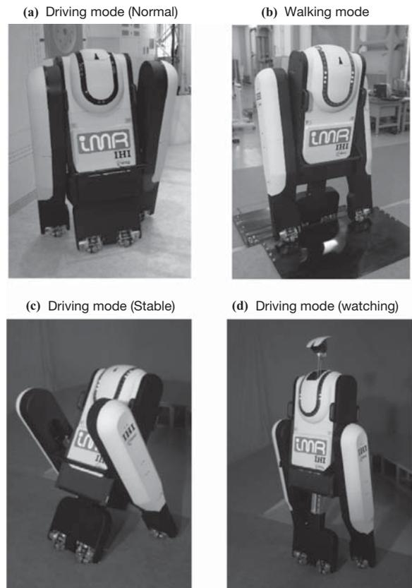
Fig. 3 Overview of Prototype Robot "IMR-Type 1"
