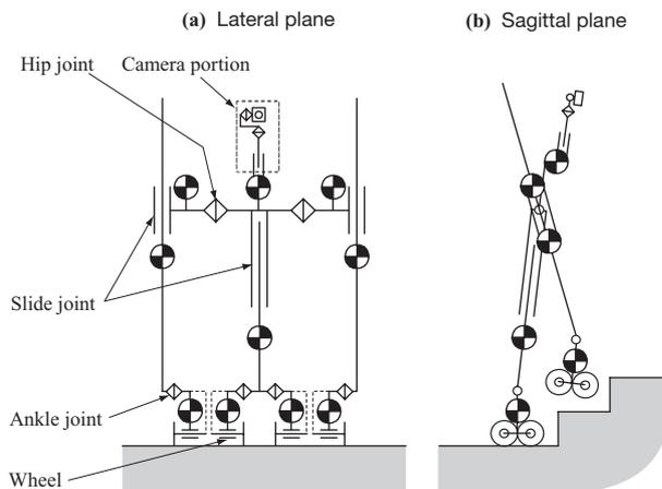
Fig. 2 Mechanical Configuration of the Robot
