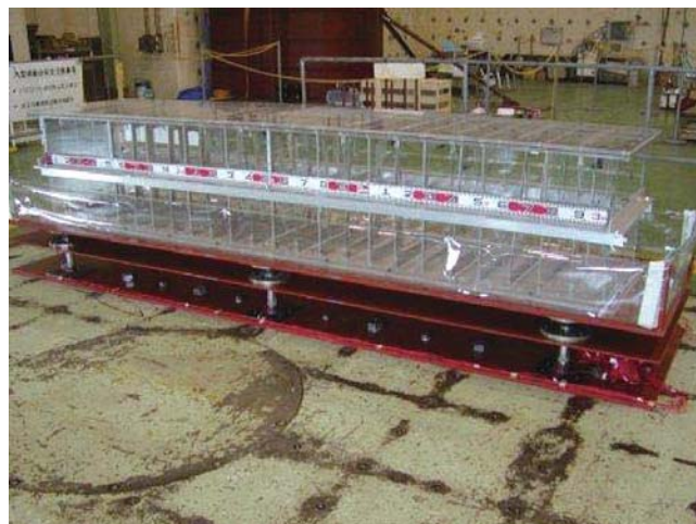
Fig. 3 Model tank for exciting test
