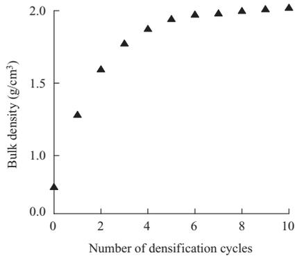
Fig. 4 Bulk density vs. number of densification cycles
