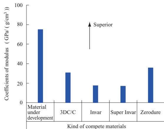
Fig. 10 Comparison of coefficients of modulus
