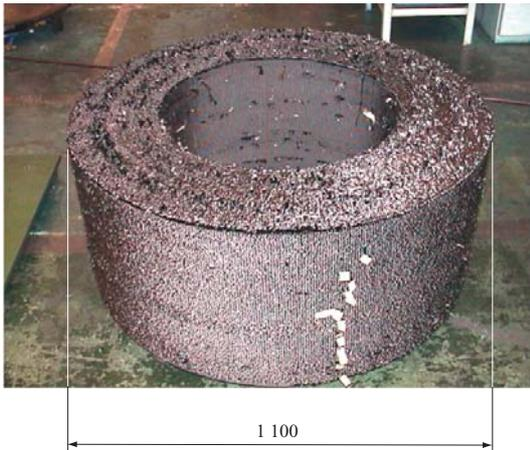
Fig. 3 3D carbon fiber preform (unit : mm)
