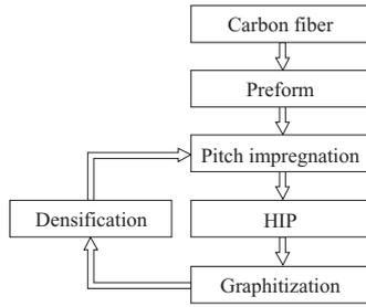
Fig. 2 Fabrication process of 3DC/C nozzle throat
