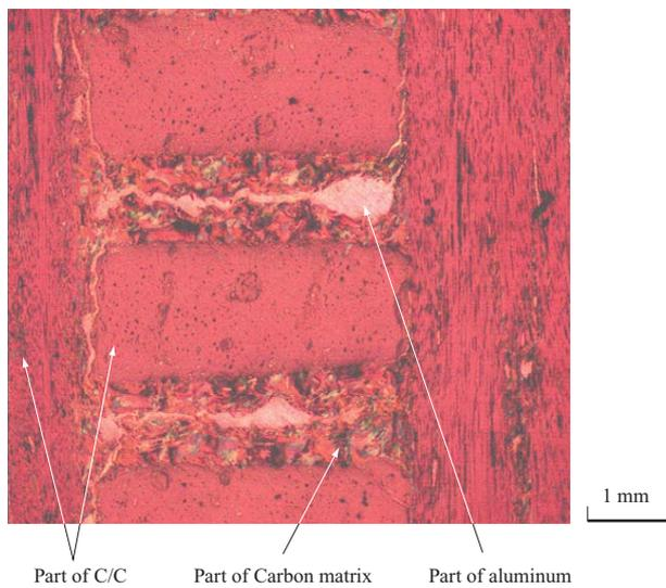
Fig. 7 Optical microstructure of 3D low C.T.E. composite
