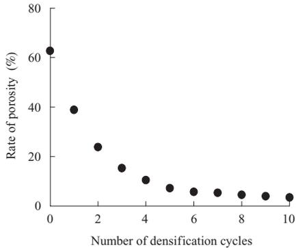
Fig. 6 Porosity vs. number of densification cycles
