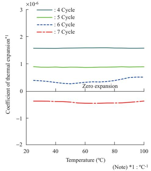
Fig. 8 Temperature dependency of C. T. E. (3D low C. T. E. composite)
