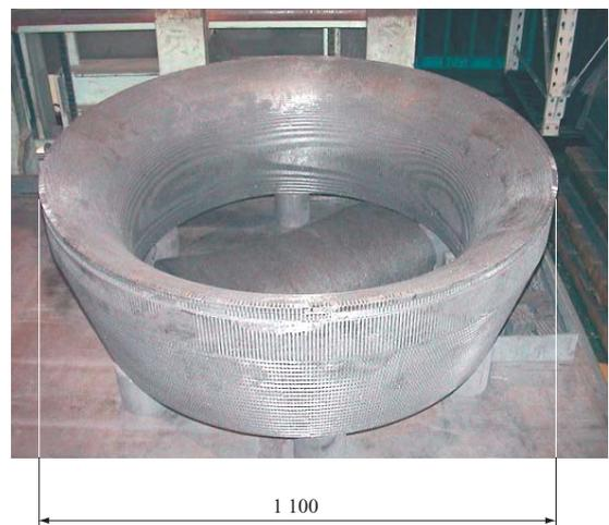
**Fig. 1** C/C composite rocket nozzle (unit : mm)
