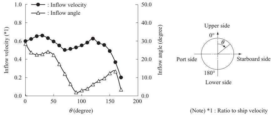
Fig. 3 Inflow velocity and angle of attack at duct position
