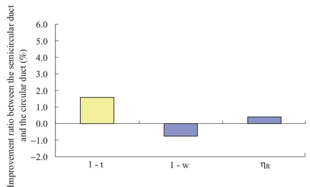
Fig. 6 Comparison of self propulsion factors between circular and semicircular ducted devices
