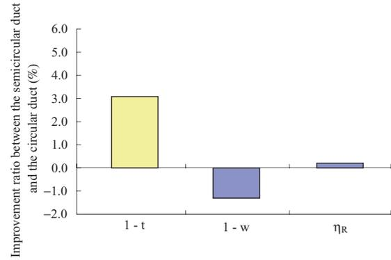
Fig. 9 Comparison of self propulsion factors between circular and improved semicircular ducted device
