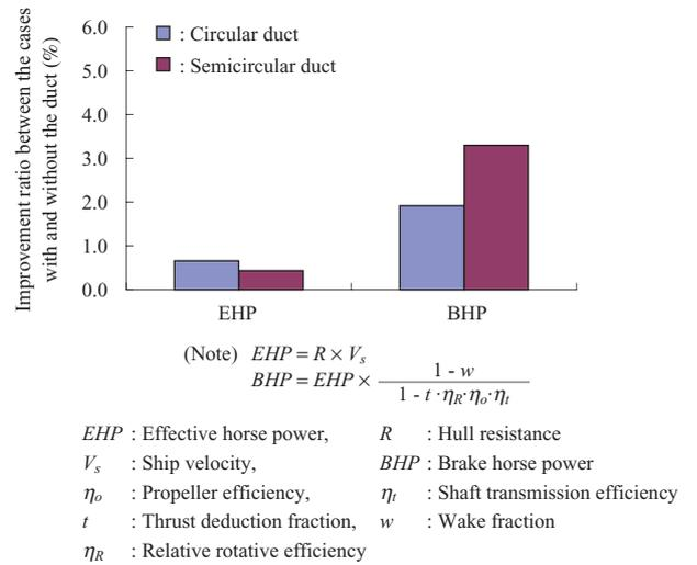
Fig. 5 Energy saving by ducted device
