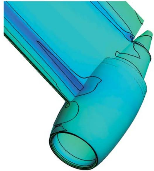
Fig. 8 CFD result of nacelle pressure distribution with pylon
