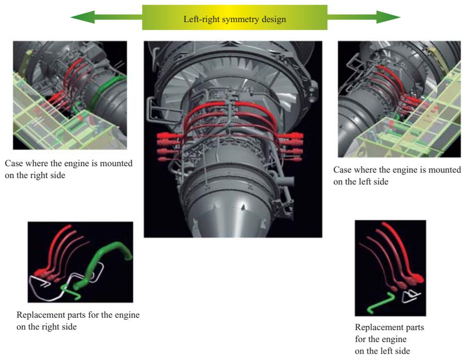
Fig. 6 Parts count reduction study of quick engine change
