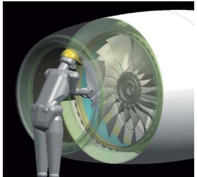
Fig. 4 Feasibility study of on-wing fan blade removal
