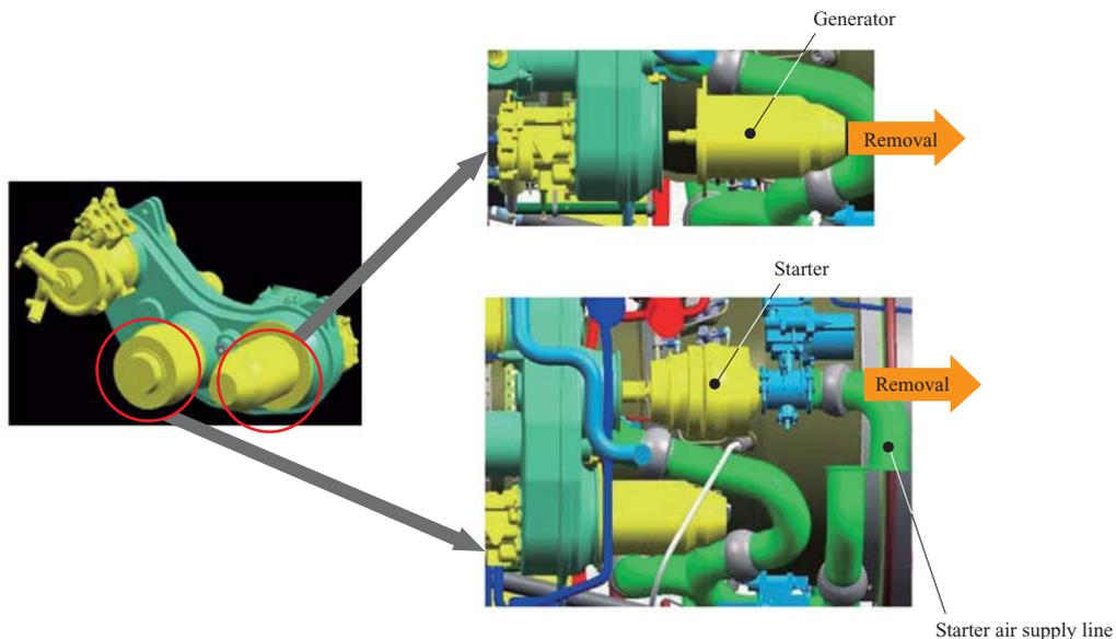
Fig. 3 Feasibility study of on-wing maintenance of line replacement unit
