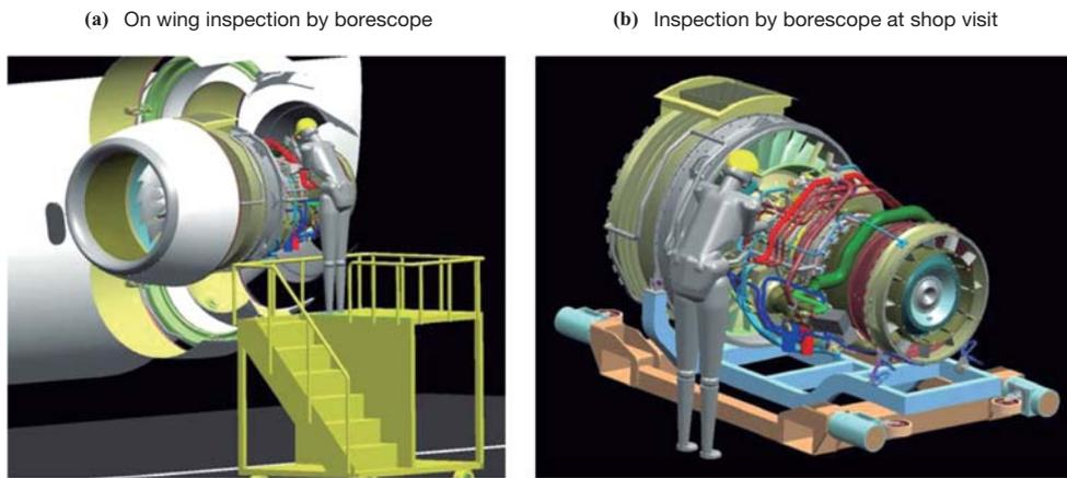
Fig. 5 Feasibility study of borescope inspection (BSI)
