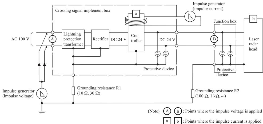
Fig. 5 Circuit of electromagnetic impulse testing
