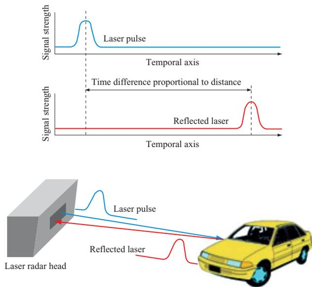
Fig. 2 Measurement principle of 3-D laser radar
