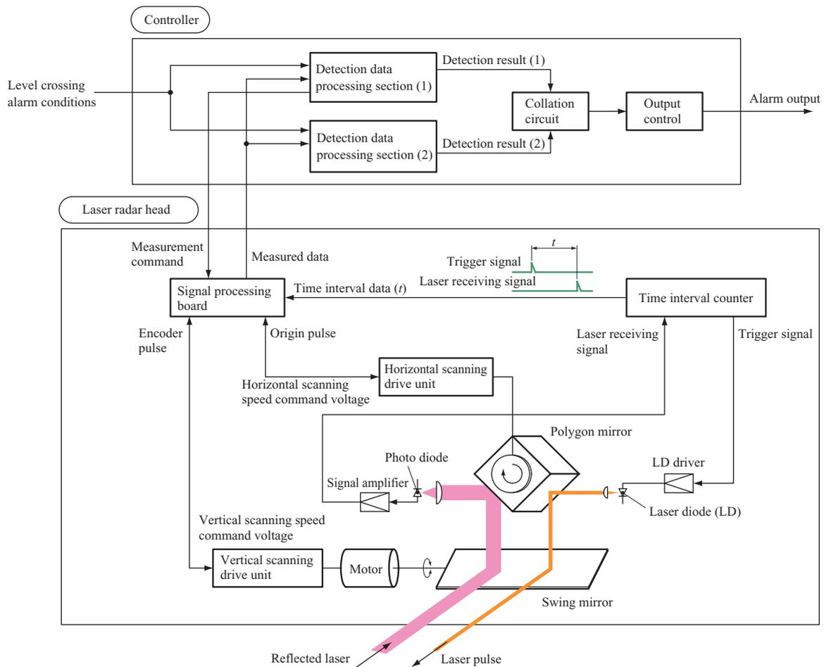
Fig. 4 Configuration of 3-D laser radar level crossing obstacle detection system
