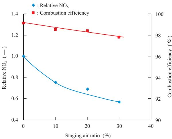
Fig. 8 Combustion characteristics ( Coal B )
