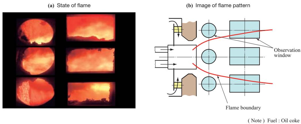
Fig. 5 Flame state using high-temperature gas recirculation burner
