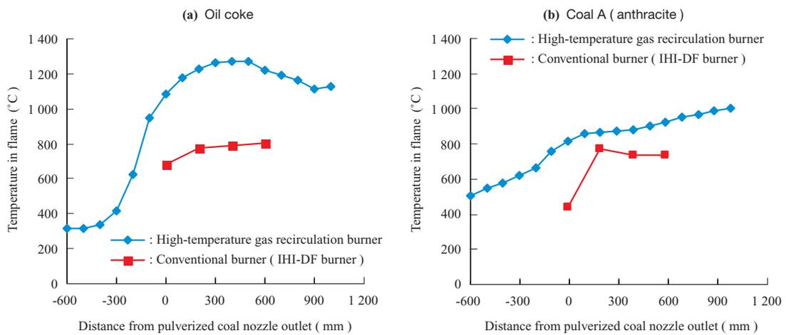
Fig. 6 Flame temperature distribution along the burner centerline
