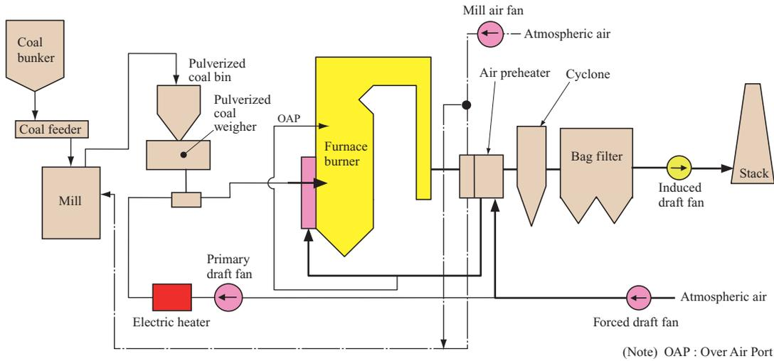
Fig. 2 Schematic diagram of combustion test facility
