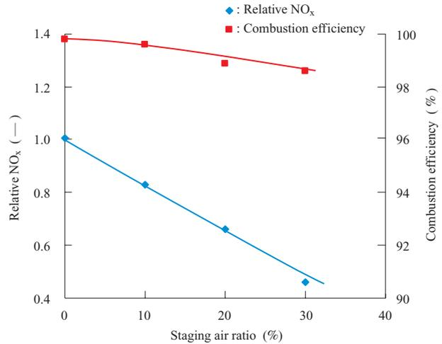
Fig. 9 Combustion characteristics ( Oil coke )
