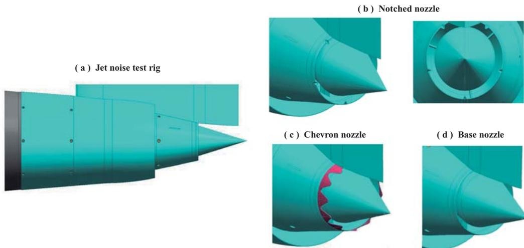
Fig. 8 Jet noise test rig with notched nozzle, chevron nozzle and base nozzle
