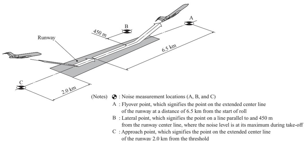
**Fig. 1** Noise measurement locations (three points) for ICAO Annex 16, Volume I, Chapter 3 regulation
