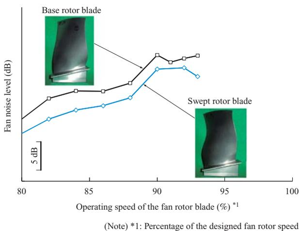
Fig. 6 Comparison of fan noise between swept rotor blade and base rotor blade
