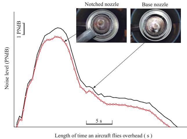
Fig. 11 Comparison of sideline noise during take-off between notched nozzle and base nozzle
