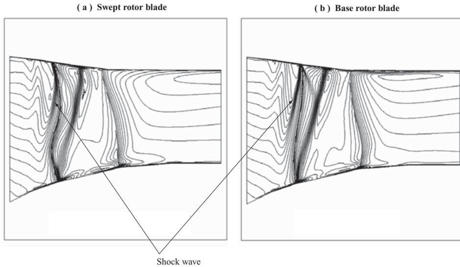
Fig. 5 Comparison of bow shock at rotor leading edge between swept rotor blade and base rotor blade (Mach contour)
