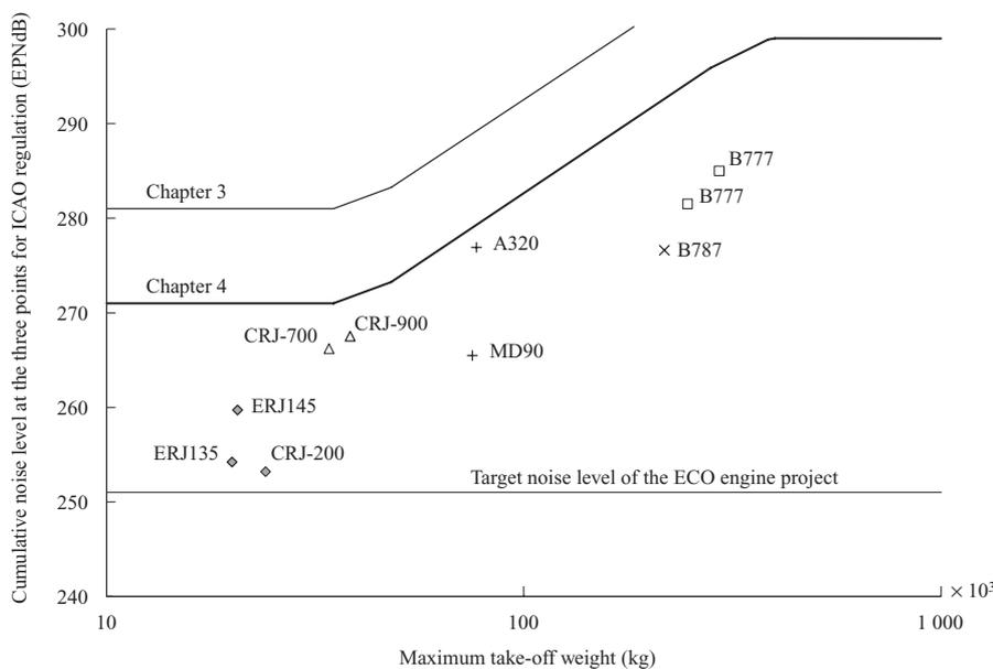
Fig. 2 Target of research and development and cumulative noise level under ICAO Annex 16, Volume I, Chapter 3 regulation
