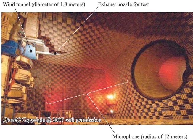
Fig. 9 Anechoic wind tunnel noise test facility at QinetiQ
