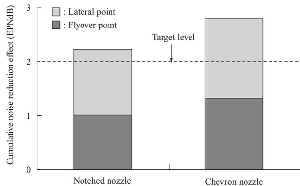
Fig. 12 Noise reduction of notched nozzle and chevron nozzle
