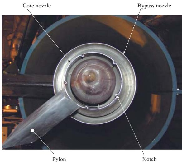
Fig. 10 Notched nozzle installed in the jet noise test rig
