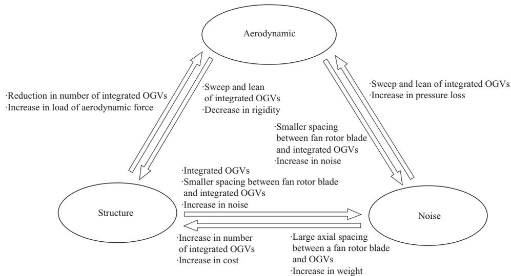
Fig. 3 Requirements and technical issues to achieve low noise maintaining low cost and low weight
