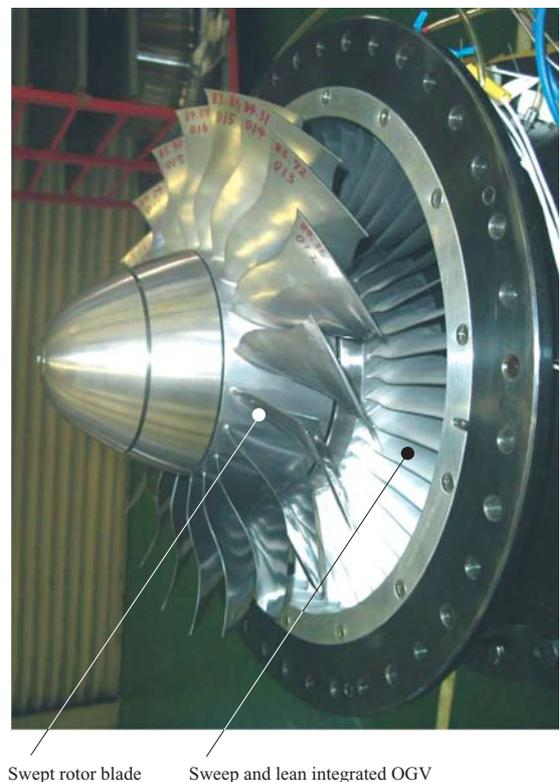
Fig. 4 Fan noise test rig
