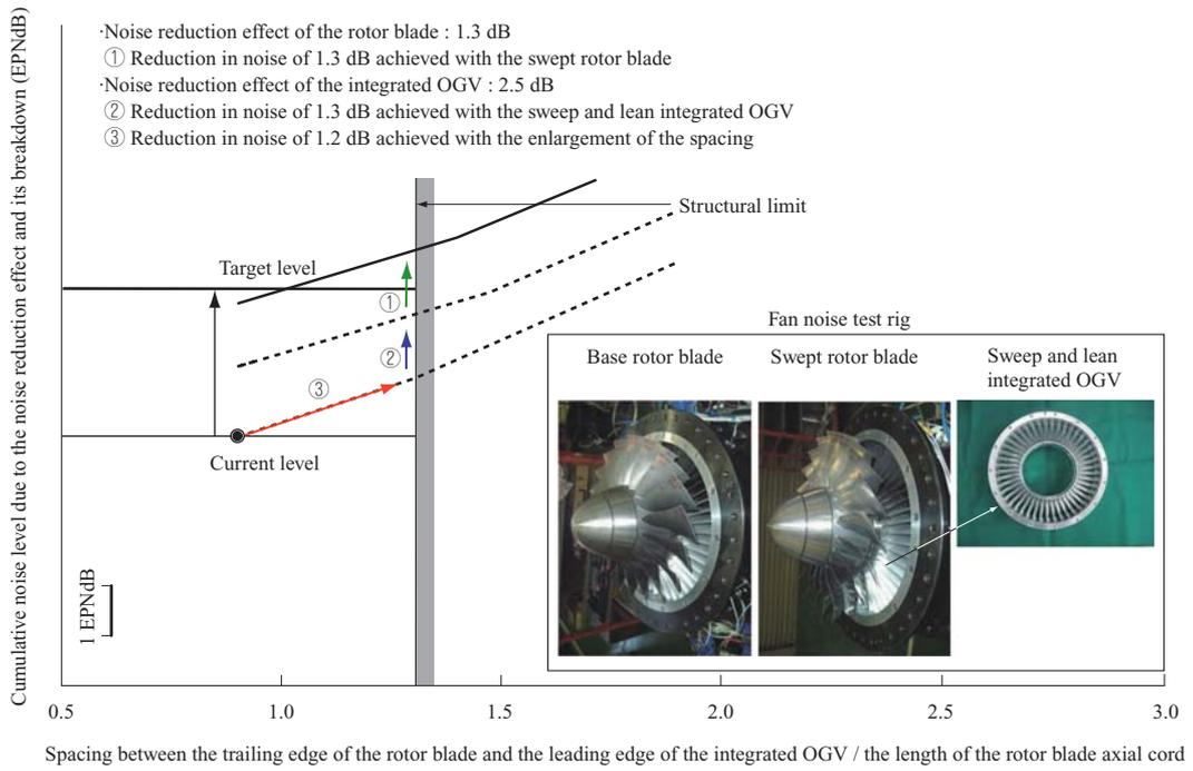
Fig. 7 Evaluation toward the fan noise reduction target
